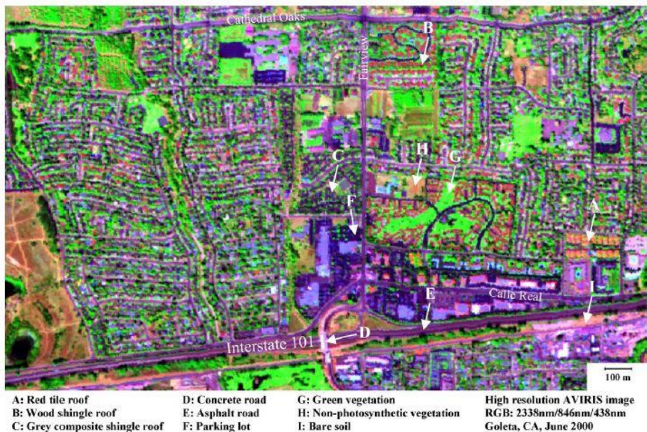
Figure 2.5. Results of remote sensing analysis to detect roof type using feature extraction of NASA Airborne Visual Infrared Imaging Spectrometer - extracted from (Herold et al., 2004)
