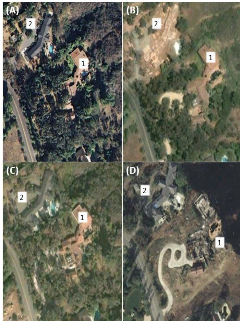
Figure 4.5. Resident response to defensible space following neighboring structure loss. Imagery taken via Google Earth in (A) March 2003, (B) June 2004, (C) January 2006, and (D) February 2008. Numbers represent specific properties.
