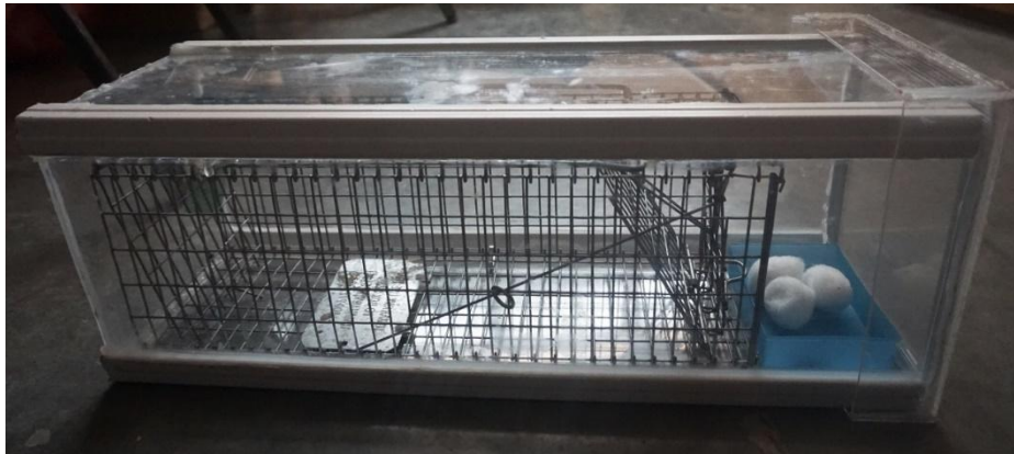
Figure 9. Plexiglas anesthesia chamber. Diagram of anesthesia chamber and lid (A) and photograph of chamber setup (B). Chamber and lid were constructed with Plexiglas, 2" corner mold, caulking and weather stripping (inner edge of lid - blue).
