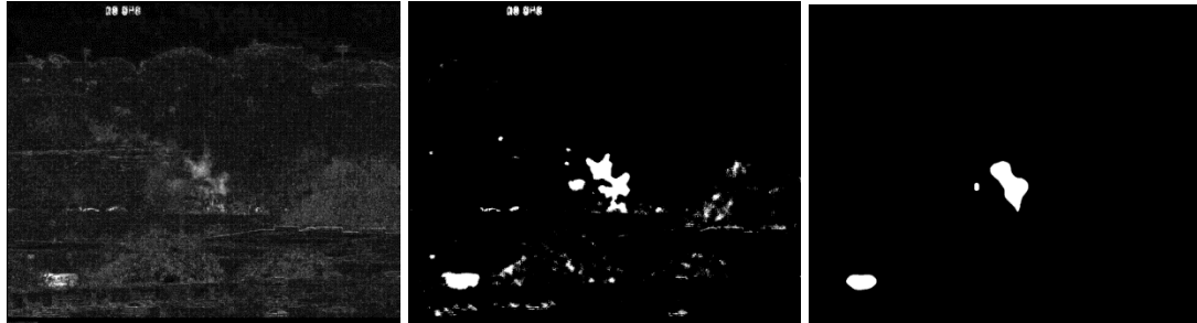
Figure 26: Difference Imaging Scheme with \Delta = 5\text{sec}
