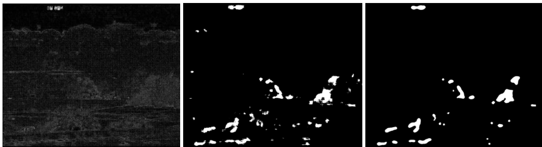
Figure 25: Difference Imaging Scheme with Delta = 2sec
