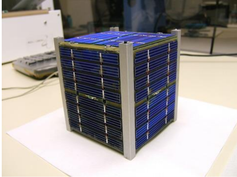
Figure 1: A 1U CubeSat Satellite prior to integration to the P-POD (CubeSat Program Pictures, 2009).
