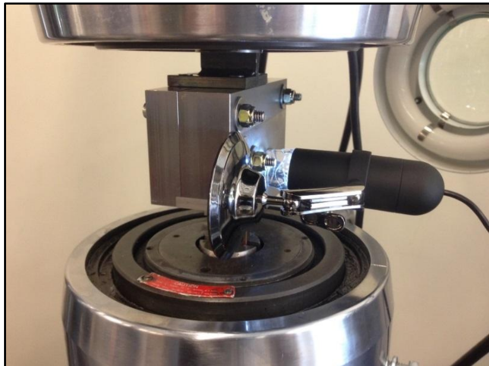
Figure 13. Digital microscope attached and aimed at anvil-tooth contact.
