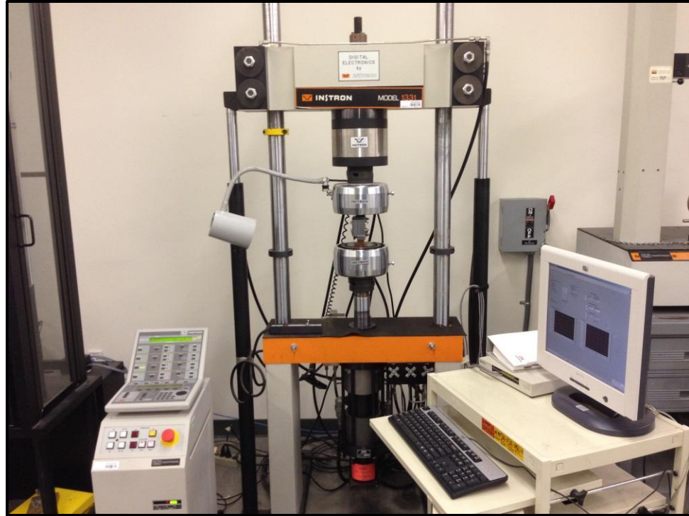
Figure 12. Overall fatigue testing test set-up.
