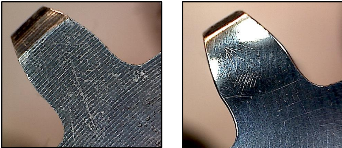
Figure 16. Gear tooth surface comparison between factory and polished surface.
