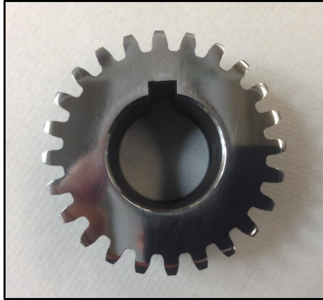
Figure 15. Gear surface after polishing.
