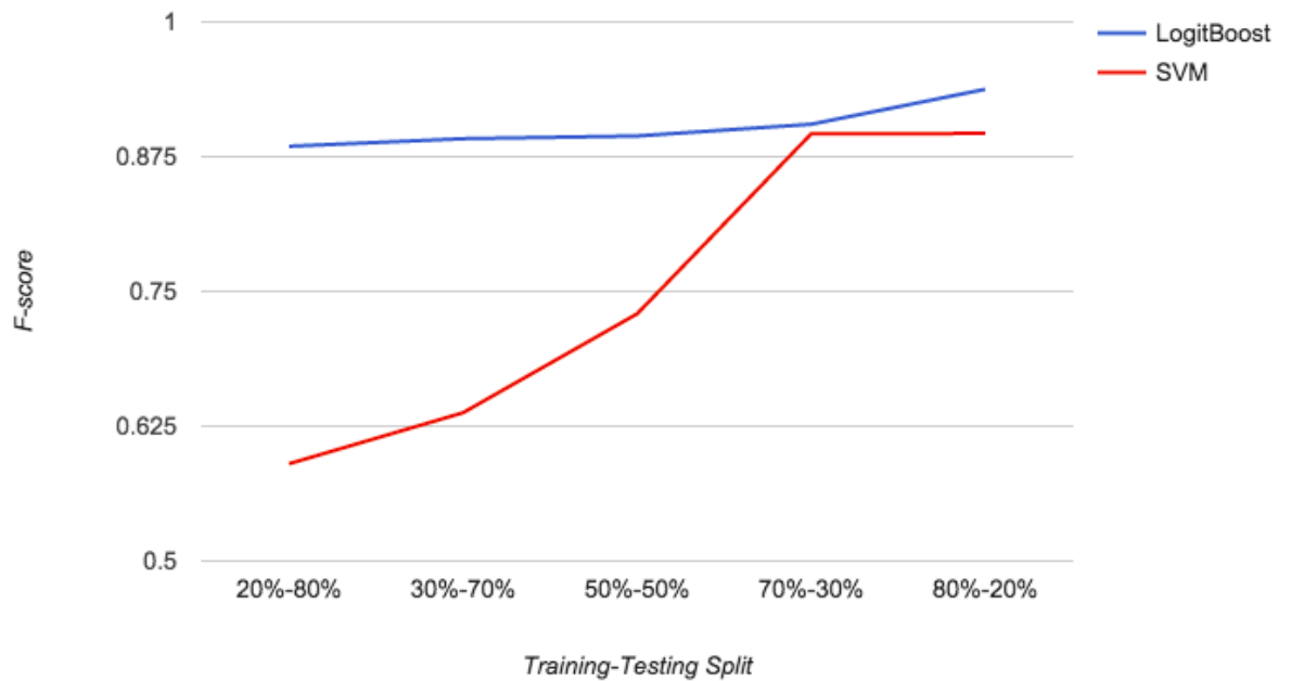
Figure 4.14: LogitBoost vs. SVM F-score: LogitBoost vs. SVM F-score. This is across each training-testing split with a total of 278 samples.
