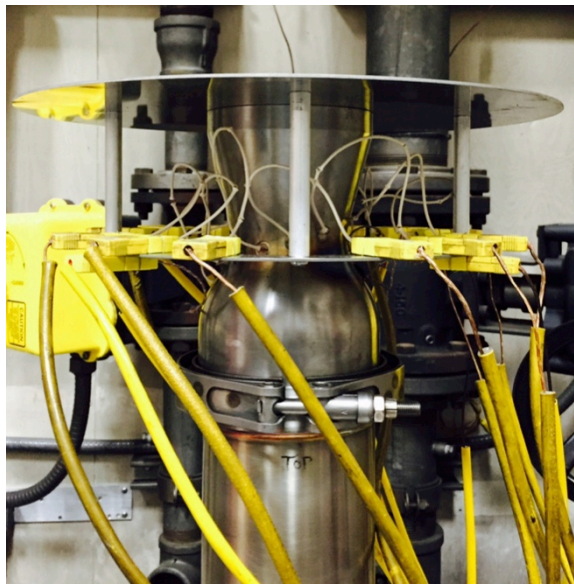
Figure 24. Complete Cal Poly 4:1 nozzle on the hybrid test stand with 18 thermocouple junctions wired to the data acquisition system.
