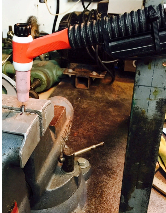
Figure 6. Thermocouple wire welding fixture. The TIG welding torch was clamped in place while the plug was fixture in a grounded bench vice with soft jaws. A special background tungsten was used to keep the arc far away from the plug wall.
