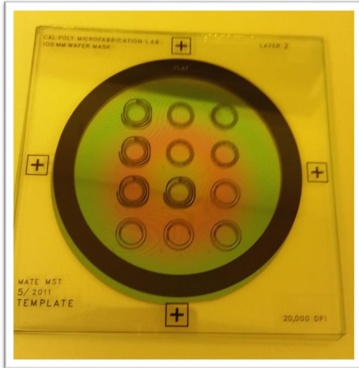
Figure 3.42 Wafer Sandwiched between Mask and Glass Slide Backing
