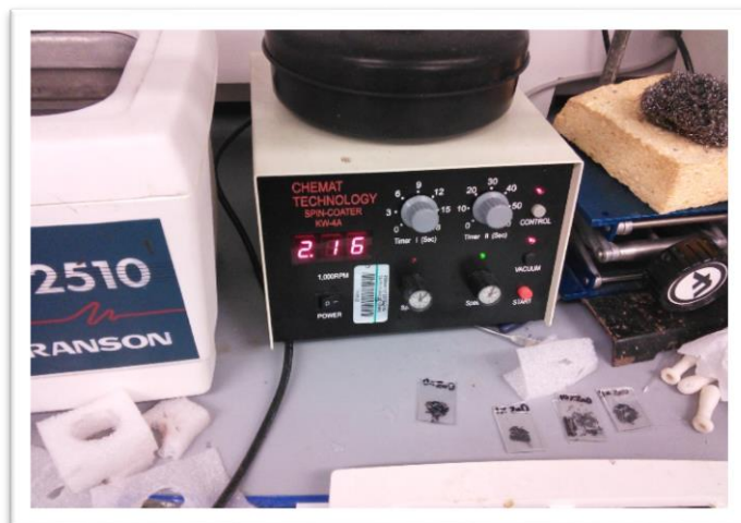
Figure 5.6 Spin Coater used to Create PEDOT Film
