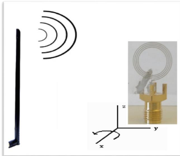
Figure 3.76 The AUT is rotated around the Horizontal Axis for Polarization Measurement
