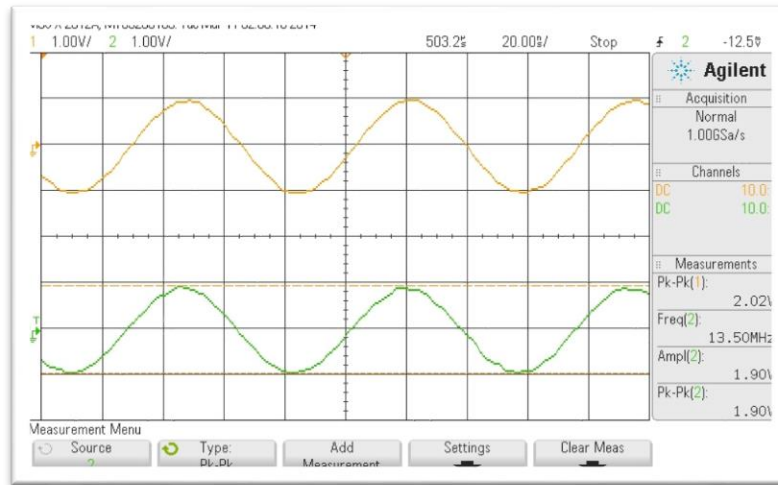
Figure 7.7 Oscilloscope Capture of Tx Signal (top) and Rx Signal (bottom)
