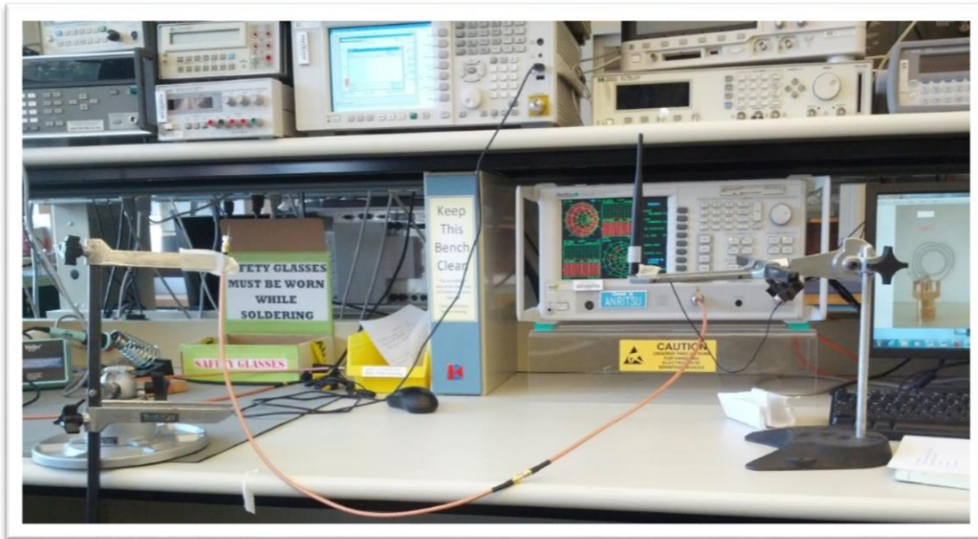
Figure 3.65 Antenna Gain Test Setup for 2.4GHz Far-Field Range of 50cm
