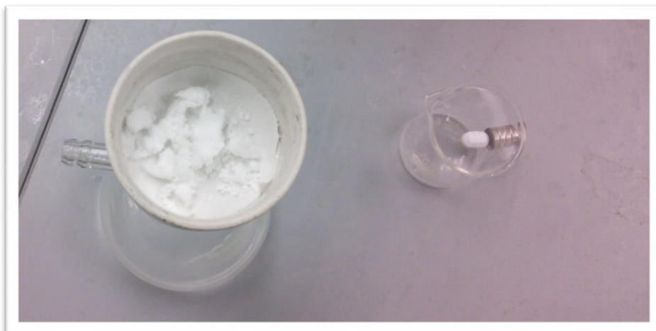
Figure 5.11 PMMA collected via vacuum filtration
