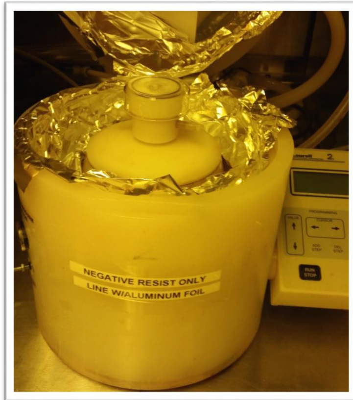
Figure 3.33 Aluminum Lined Spin Coater
