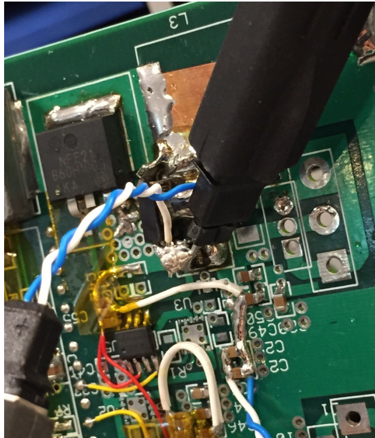
Figure 9-30: Method used to measure voltage across the current sense resistor with differential probes of Two Phase PWM Converter
