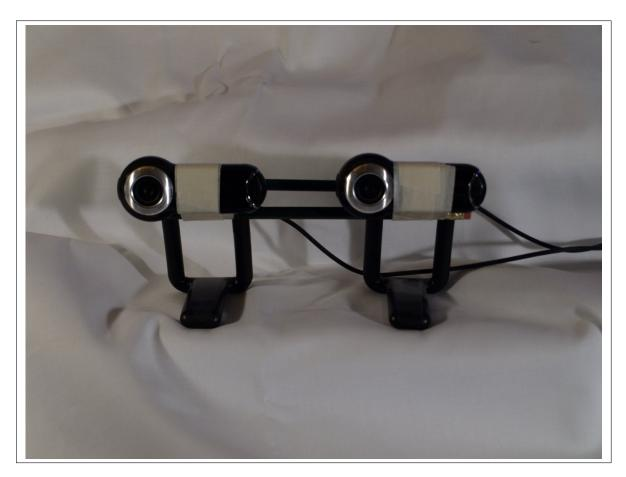
Figure 4.1: A stereo camera rig built out of two web cams, masking tape, and pencils.
