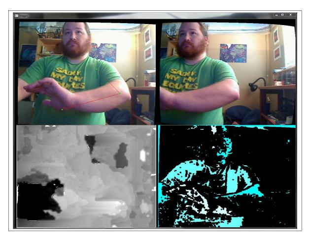
Figure 4.2: An example from the system, showing the depth map and tracked arm.
