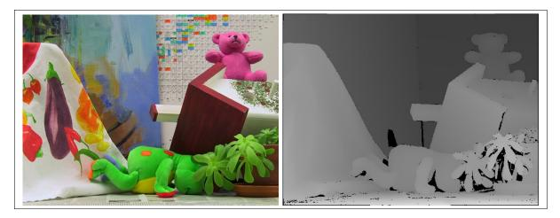
Figure 2.7: An example of a depth map. A. One of the images from the stereo pair. B. The extracted depth map. Images from [2].
