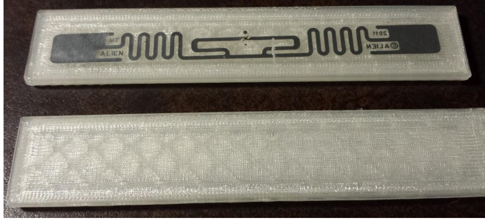
Figure 6- RFID inlay and unconnected substrate halves
