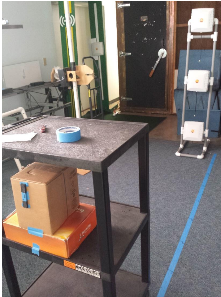
Figure 8- Experimental Setup: cart, measurement/guide tape, and antenna
