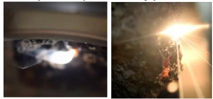
Figure 9. Right photo was taken during a low pressure ablation test and shows mass ejecta and plume. Left photo was taken during an ablation test at ambient pressure and shows the sample smoking and melting.
