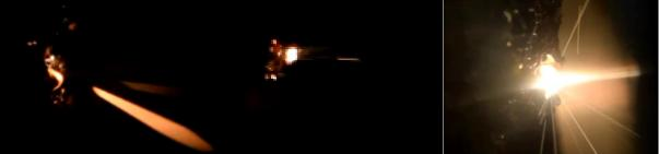
**Figure 16.** Various pictures of mass ejecta, sparks, plume, and bubbles due to laser ablation. These pictures show the environment at the sample while laser ablation is occurring. See online video.
