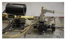
**Figure 10.** Ablation laser directed at the Power Meter. Power meter was used to determine the slope efficiency of the ablation laser up to 20 amps.
