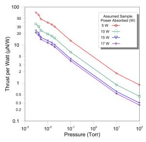
**Figure 15.** Momentum Coupling Coefficient for various assumed power absorbed by sample. Each line represents a different power **absorbed** by the sample for 20W at outside lens.
