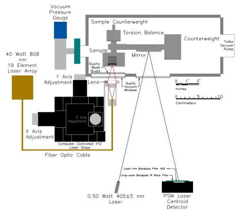
**Figure 3.** Top-view model of experimental setup. Ablation laser feeds through a fiber optic cable, through a lens, and past 2 quartz windows to ablate the sample on a torsion balance. As the torsion balance rotates the measurement laser reflects off a mirror and moves along the PSM.
