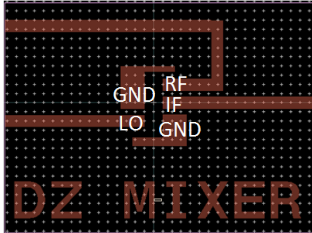
Figure 3.9 ADE_42MH mixer matching circuit layout
