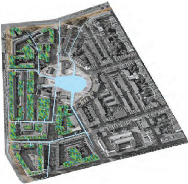
Figures 3 a & b: Rotterdam's Water Square, 2010: collection of the neighborhood's storm water and retention in a multifunctional park. (courtesy: De Urbanisten, Florian Boer, Jens Jorritsma, and Dirk van Peijpe; photo by Maria Matos Silva)
