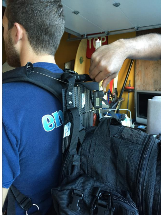
Figure 29. Measuring distance between plates to determine force in springs.
