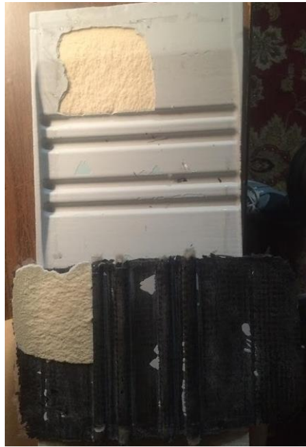
Figure 25. First attempt at pulling composite part off of mold.
