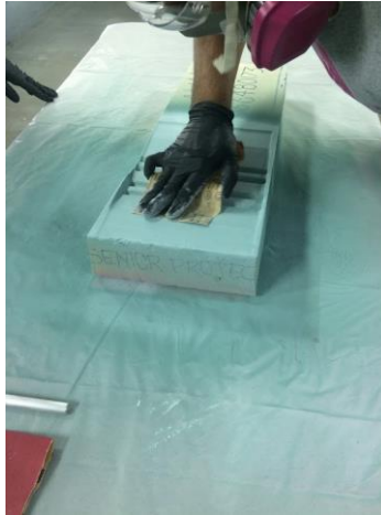
Figure 23. Sanding the mold between layers of Duratec.
