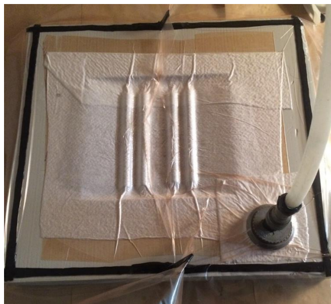
Figure 26. Vacuum bagging process for laminate curing.
