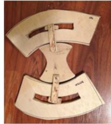
Figure 12. Three panel pivot sketch (left) and wood prototype (right).
