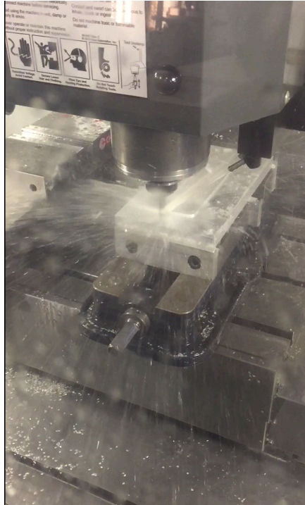
Figure 8-3: CNC Machining of the main structural Bracket in the IME Lab on a Haas CNC
