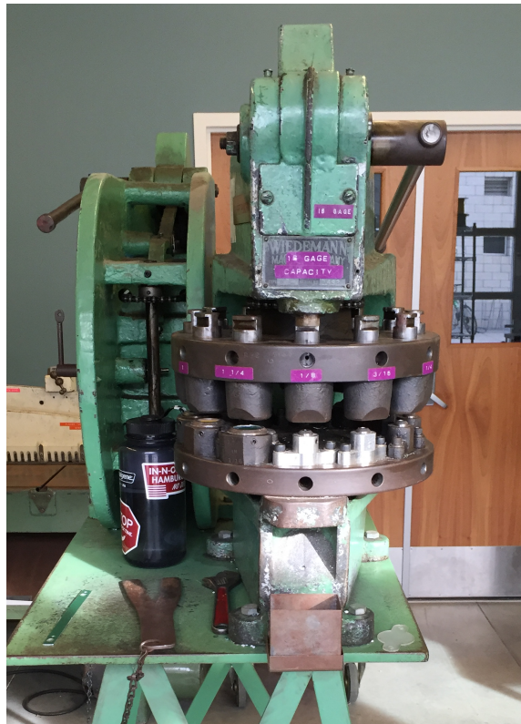
Figure 8-5: Hole punch available in the IME metal working lab used to create the limit switch l-bracket
