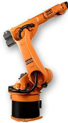
Figure 2-2: Kuka KR30-3 Robot 3
