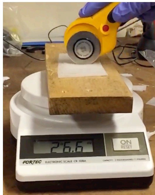
Figure 4-7: Cutting Force Testing Rig (lbf)
