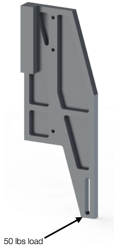
Figure 5-14: Design load for bracket design
