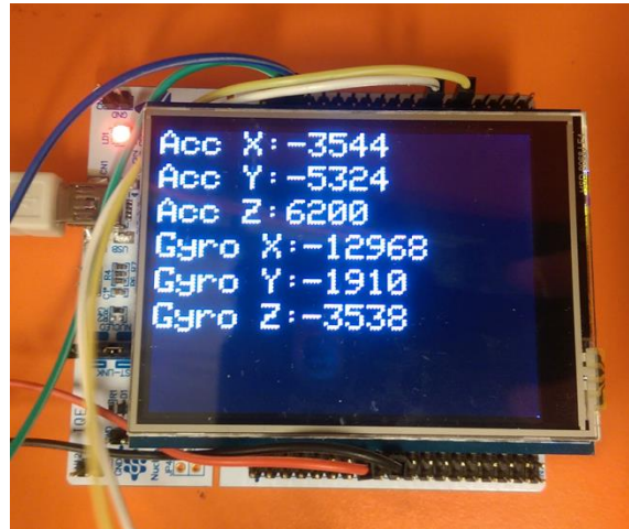
Figure 6: Example of program running and displaying sensor data
