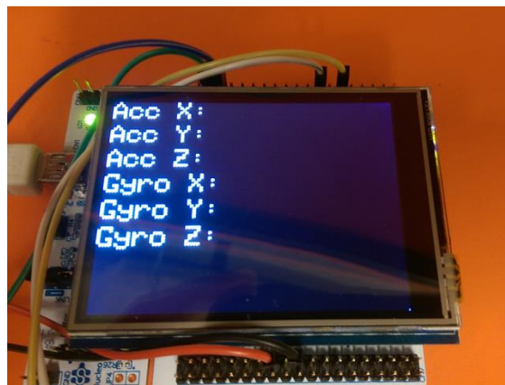
Figure 5: Initialization of screen before reading sensors
