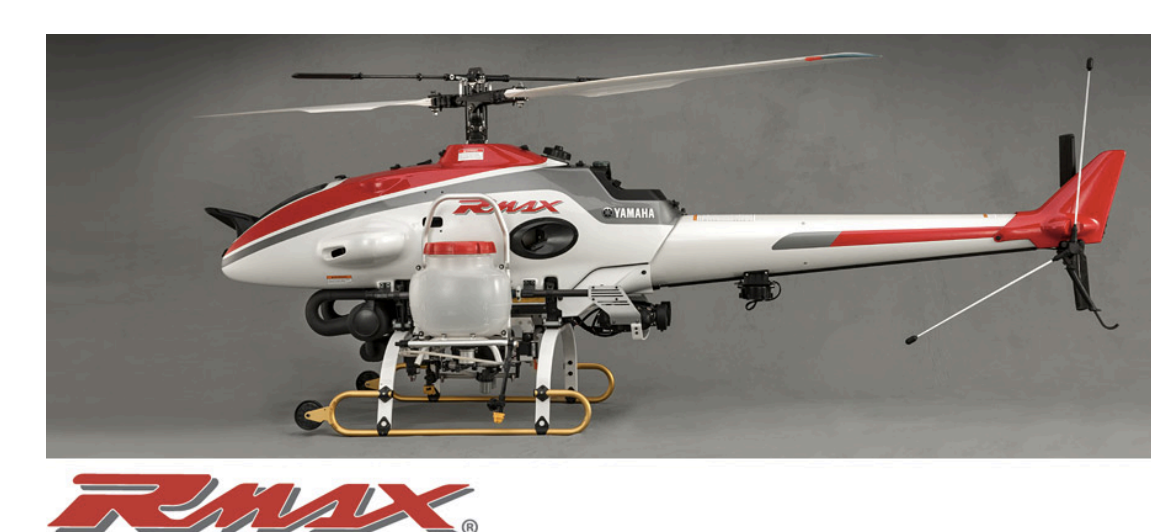
Figure 3: Yamaha R-MAX is a two-bladed, gasoline-powered, unmanned helicopter Rotor Diameter: 10' 3" Length: 11' 11"
