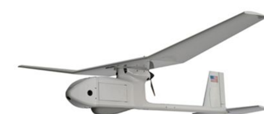
Figure 2: AeroVironment RQ-20 Puma is a small, battery powered, hand-launched UA. Wingspan: 9' 2" Length: 4' 7"
