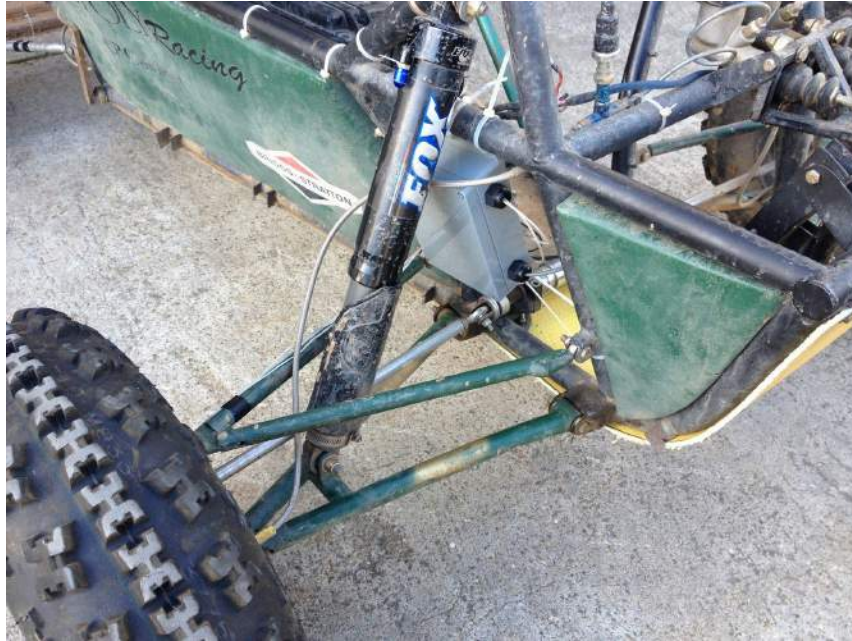
Figure 45. Spindle Strain Gauge Amplifier Location
