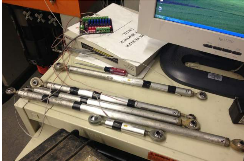
Figure 52. Rear Link Amplifier Offset Calibration Process (Off-Car)
