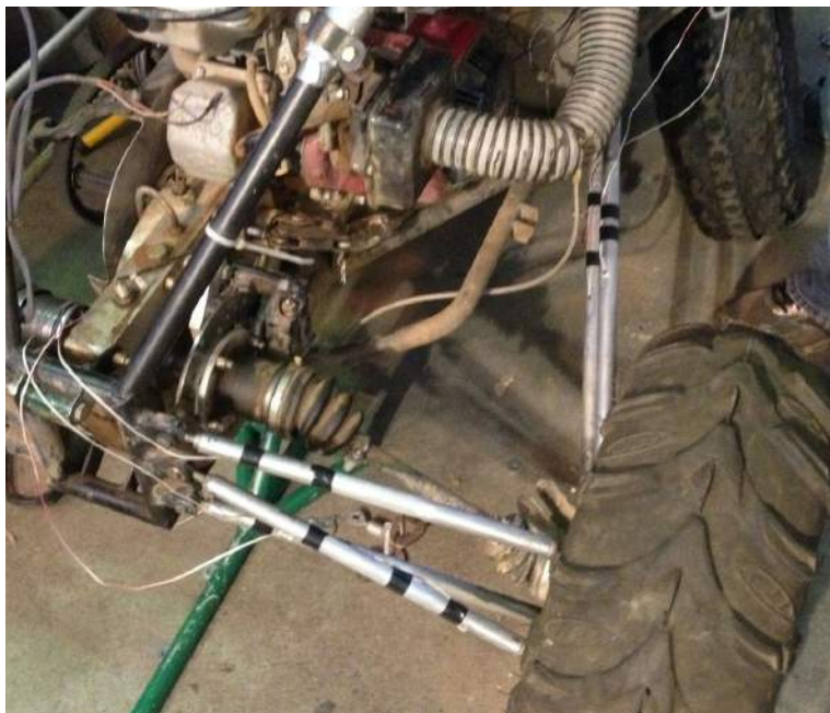
Figure 50. Rear Links Strain Gauge Wiring and Assembly
