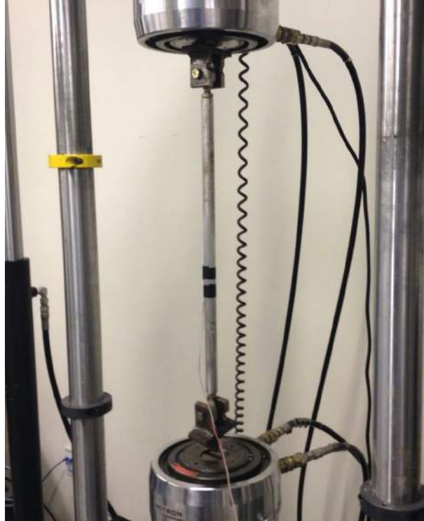
Figure 56. Rear Link Clevises and Instron Calibration Testing
