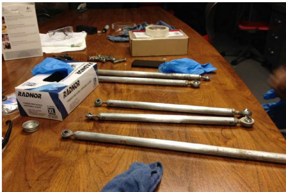
Figure 49. Prepped Axial Links for Strain Gauge Application
