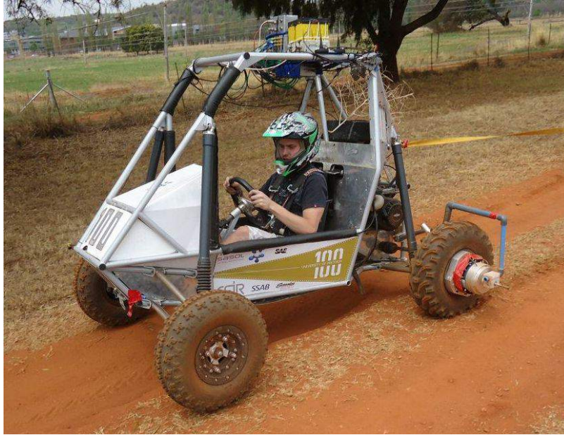
Figure 22. University of Pretoria in South Africa's Custom Wheel Force Transducer
