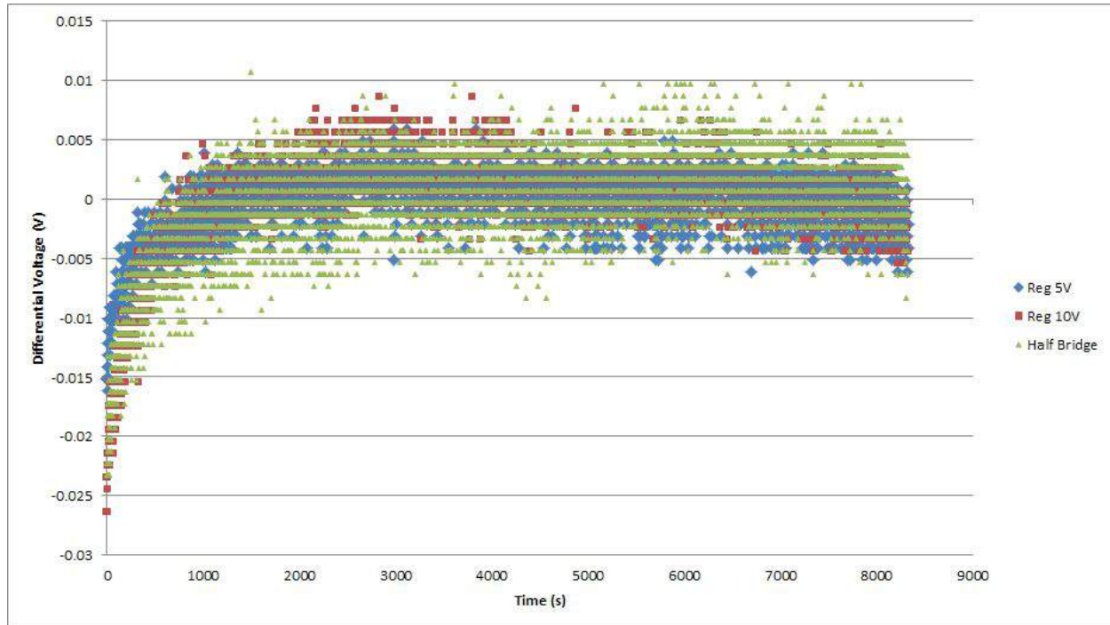
Figure 61. Controlled Temperature Test: Unstressed Half Bridge
