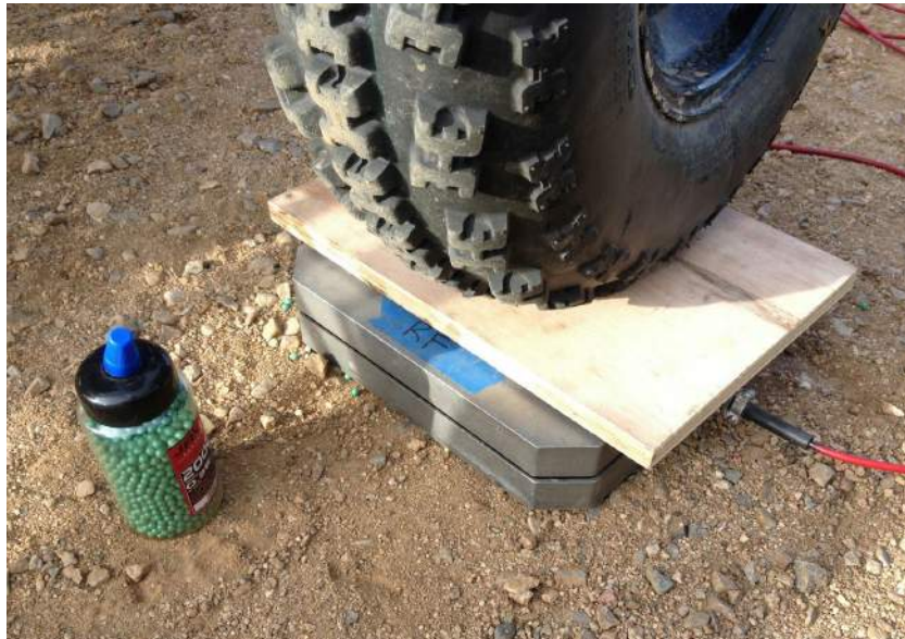
Figure 58. Removal of Induced Side Forces with Suspension Travel using Plastic BBs as Rollers
