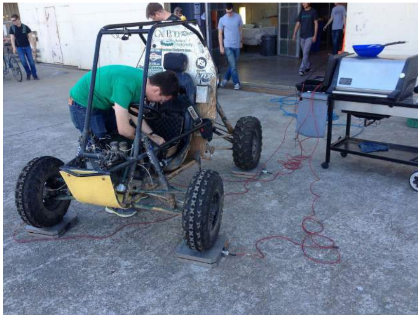
Figure 57. Attaching the DAQ and Recording Weight of Vehicle on Car Scales
