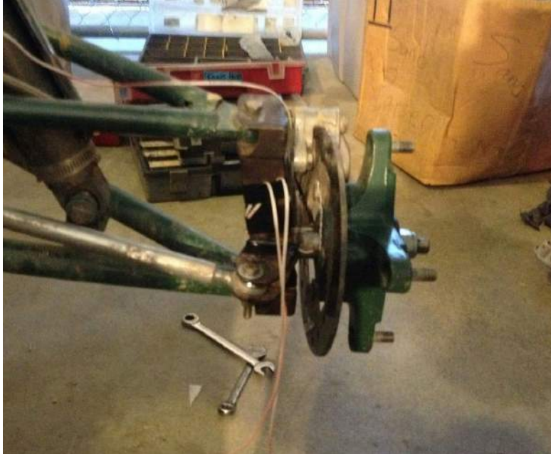
Figure 51. Front Spindle Strain Gauge Wiring and Assembly
