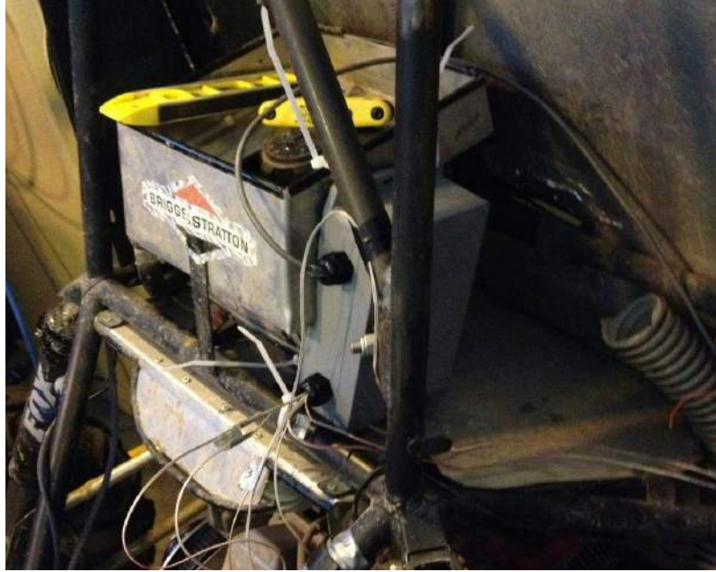
Figure 46. Rear Links Strain Gauge Amplifier Location
