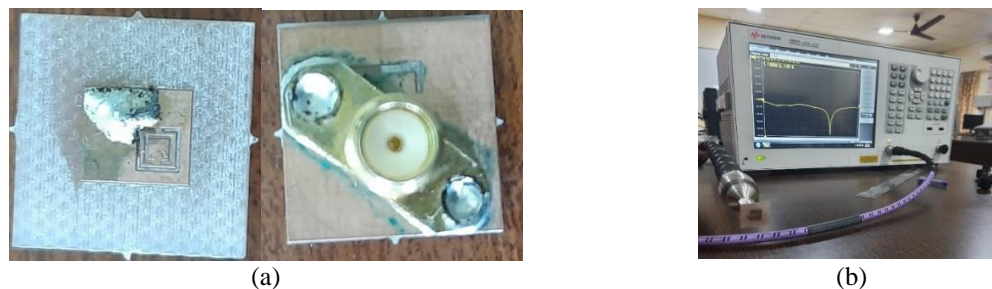
Figure 8. Realized antenna and measurement setup, (a) Realized antenna, and (b) Antenna measurement using VNA
