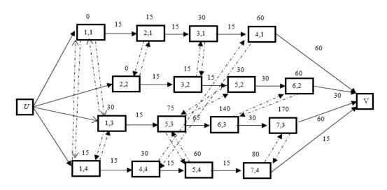
Figure 2. Disjunctive graph of proposed JSS model
