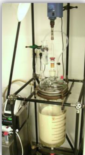
Figure 6. Scaled up desymmetrization of dimethyl cyclohex-4-ene- cis -1,2-dicarboxylate; left: temperature controlled bioreactor with a total capacity of 10 L; right: time course of concentration of reagent 1 (■), concentration of product 2 (□) and ee (●) as determined by GC analysis; Conditions: 200 mM substrate, 5.5 U/mL ECS-PLE06, total volume: 8.8 L, stirrer speed: 300 rpm, 40°C, pH control via acid scavenger NaHCO 3 .
