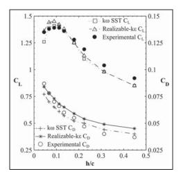
**Figure 4.** Drag coefficients and lift coefficients: comparison of the validation cases with the experimental results. SST: shear stress transport.
