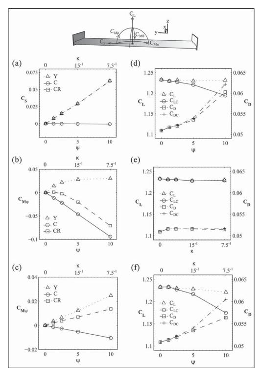
**Figure 12.** Aerodynamic force and moment coefficients acting on the wing: (a) side-force coefficients; (b) rolling moment coefficients; (c) yawing moment coefficients; (d) lift coefficients and drag coefficients for cases Y; (e) lift coefficients and drag coefficients for cases C; (f) lift coefficients and drag coefficients for cases CR.
