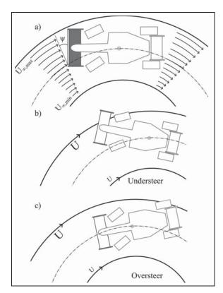
**Figure 2.** (a) The cornering flow conditions; (b) the effect of understeer toward the flow seen by the front wing; (c) the effect of oversteer toward the flow seen by the front wing.
