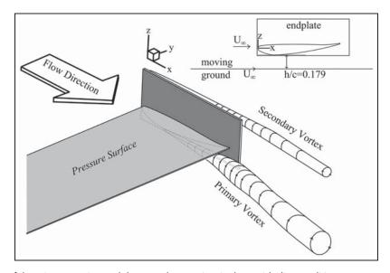
Figure 1. Location of the primary vortices and the secondary vortices in the straight-line condition.
