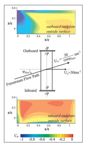
**Figure 6.** Change in the pressure occurring near the endplates owing to the flow angle and the pressure coefficient contours over the outside of the endplates for case Y4.
