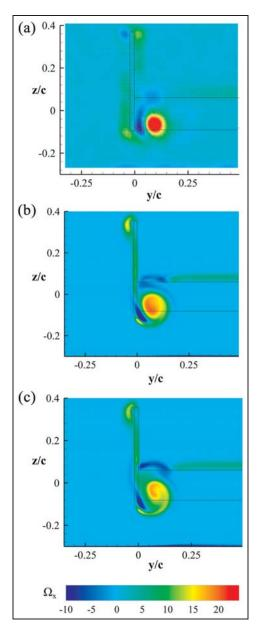
**Figure 5.** Streamwise vorticity contours for h/c = 0.224 at x/c = 1.2: (a) experimental; <sup>12</sup> (b)  $k-\omega$  SST; (c) realizable  $k-\varepsilon$ .
