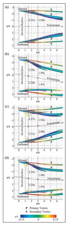
**Figure 10.** *Q* criterion of 20 000, indicating the primary and secondary vortex paths which are colored according to the proximity of the ground: (a) case S; (b) case Y4; (c) case C4; (d) case CR4.
