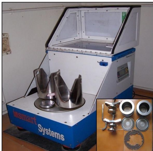
Fig. 1 – Twin-bowl type planetary ball mill system. Inset figure shows the tungsten carbide (WC) lined stainless steel vial and WC balls
