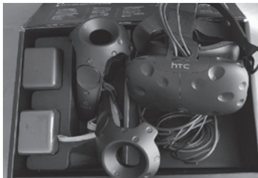
Figure 6: HTC Vive technology basic setup
