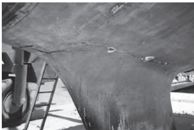
Figure 1: A large crack as a result of hard grounding [13]
