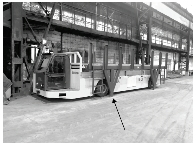
Figure 1 The electric transporter with blue cassette [1]
