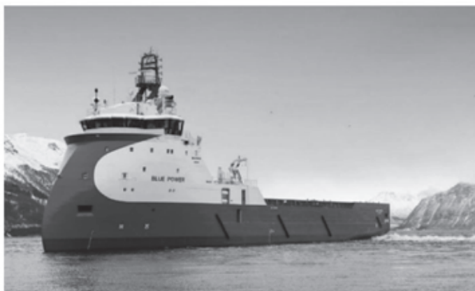
Figure 5: Platform supply vessel Ulstein PX121 [3].
