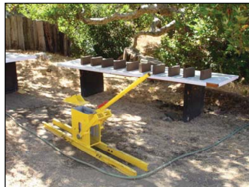
Figure 2: Hand brick press and bricks air curing.
