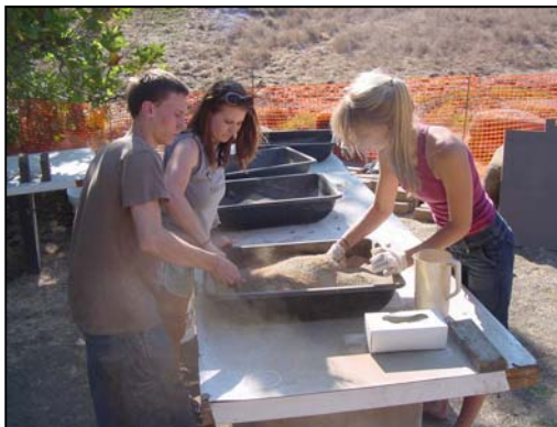
Figure 1. Students measuring and mixing dry materials of adobe mix.
