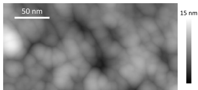
Fig. 9 – Tip convolution simulated by a dilation algorithm on the data in Fig. 7
