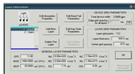
Fig. 2 – AMPS simulation front panel contains the device and layer grid parameters, and general layer parameters
