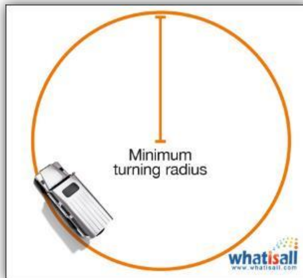
FIGURE 69. DIAGRAM DEFINING TURNING RADIUS FOR A VEHICLE. (WHAT IS TURNING RADIUS?, 2012)
