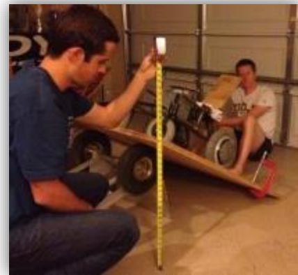
FIGURE 62. FRANKIE MEASURING THE TILTOVER HEIGHT.
