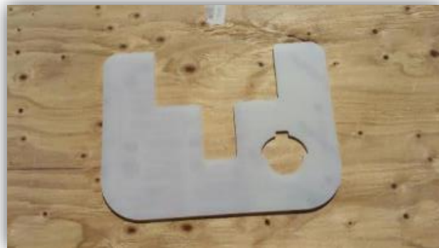
FIGURE 32. NEW POLYCARBONATE ARM REST WITH ANTI-SCRATCH PROTECTIVE SHEETING ON IT.
