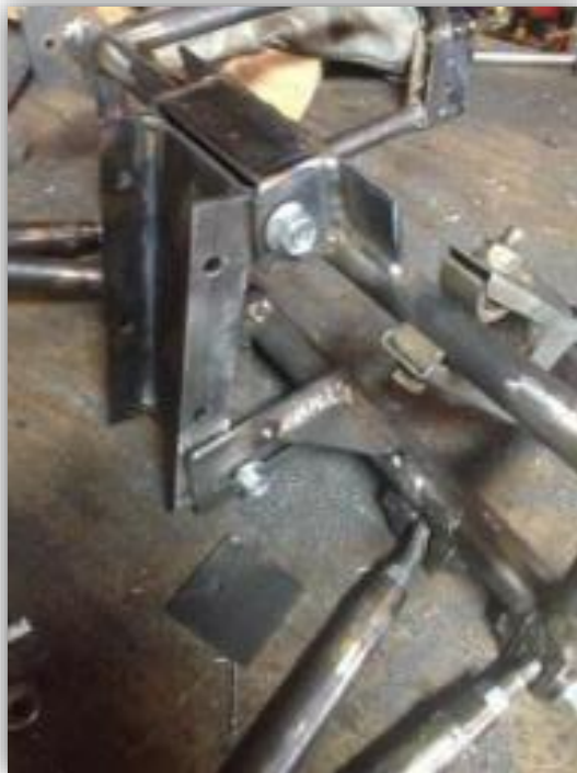
FIGURE 50. CENTER COLUMN MOUNTING PIECE ATTACHED TO OUR FRAME.
