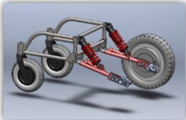
FIGURE 30. TRAILING ARM ATTACHED TO FRAME AND SHOCK.
