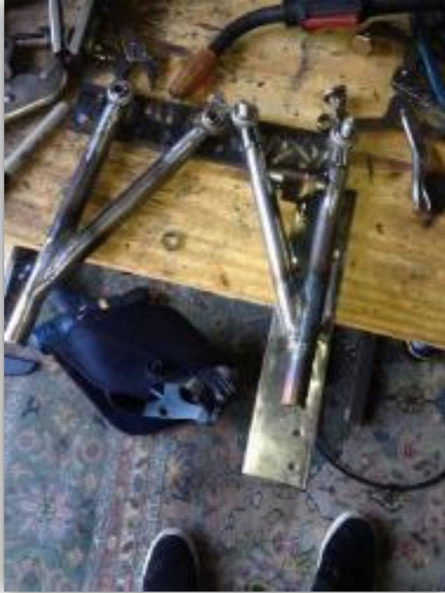
FIGURE 45. FIXTURES TO CREATE IDENTICAL TRAILING ARMS.
