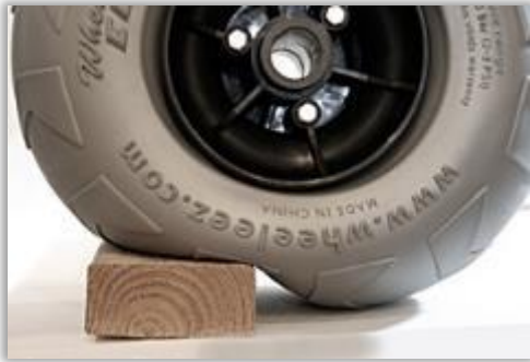
FIGURE 17. LOW PRESSURE TIRE DEFLECTING AROUND A 2X4 WOODEN BEAM. (DEFLECTION OF TIRE, N.D.)
