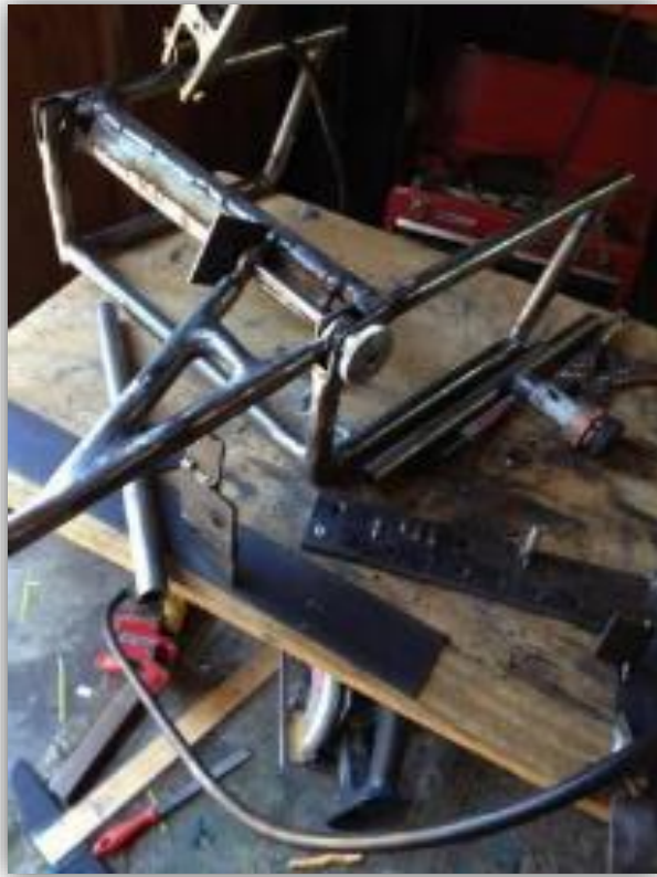
FIGURE 47. ATTACHING OUR TRAILING ARM TO OUR TEST RIG.
