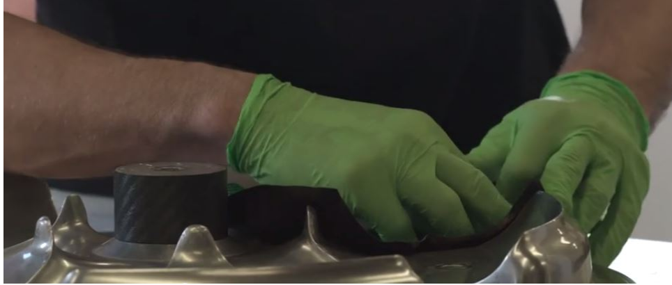
Figure 5: The Aircore wheel being made by hand layup in an aluminum mold 14 .
