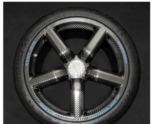
Figure 4: The Koenigsegg "Aircore" wheel. A hollow CFRP structure weighing a total of 13lbs 15 .
