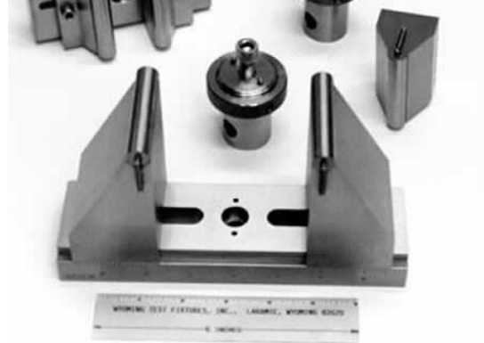
Figure 12: Wyoming Test Fixtures flexure testing setup 27 .
