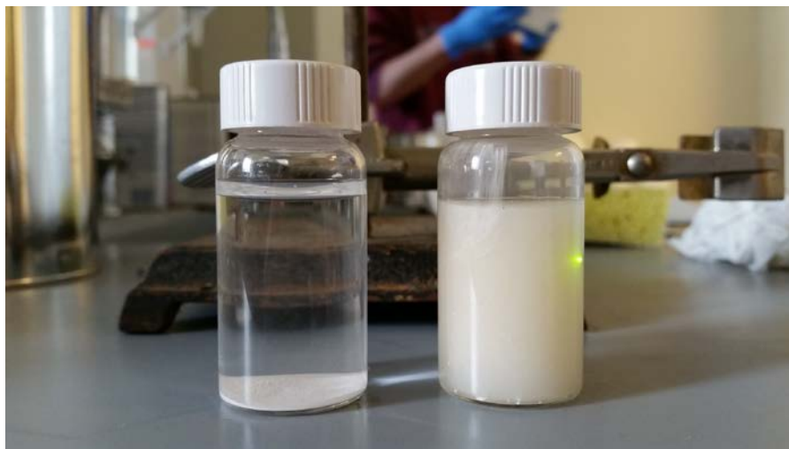
Figure 3: A comparison of taggants in DI water (left) and 3 wt.% HEC (right) after 10 minutes.
