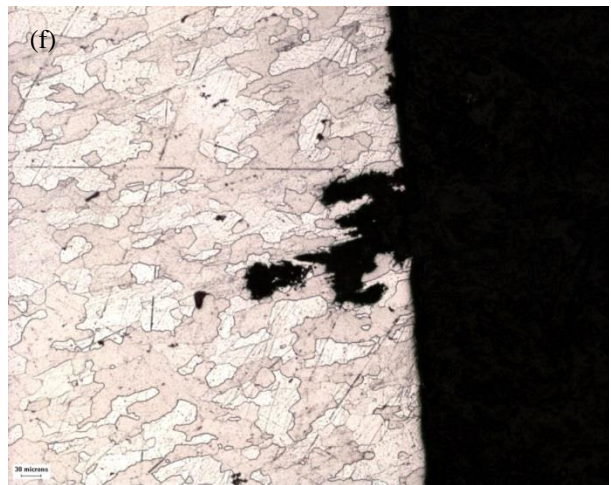
Figure 23– 4 hour solution heat treatments at (a) 890°F, (b) 900°F, (c) 910°F, (d) 920°F, (e) 930°F, and (f) 940°F. Immersed in a H 2 O 2 and NaCl solution for 6 hours and then prepared metallographically. Small varied amounts of pitting at the surfaces but no signs of intergranular corrosion.
