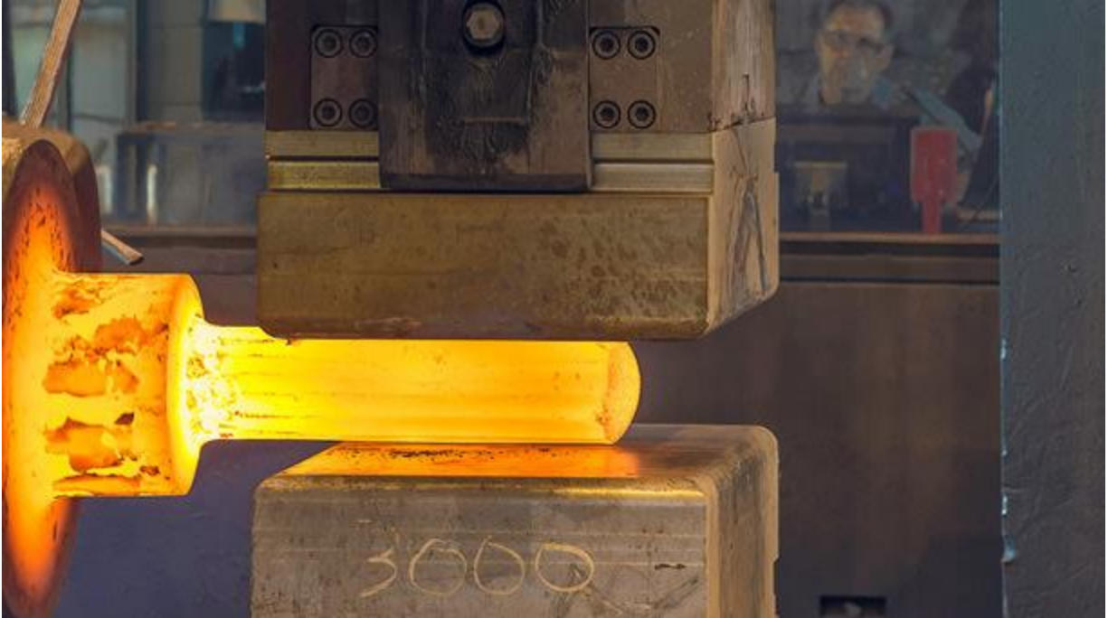
Figure 4 – A Scot Forge crew forges a steel journal down to size on a 3000 ton hydraulic press. A crew of four, including a forge operator, blacksmith, forklift operator, and manipulator operator work on each press at any given time. [9]
