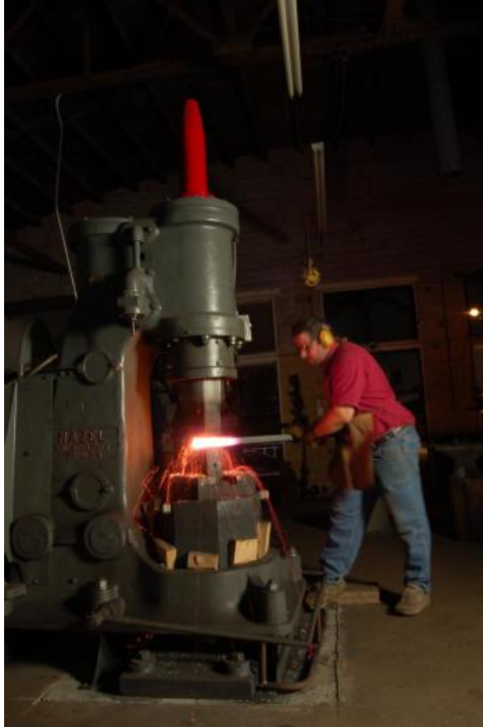
Figure 3 – A blacksmith forges steel on his Nazel 3B power hammer. Even though it is an energy restricted machine, the amount of force can be controlled by the position of the work piece within the stroke length. [8]
