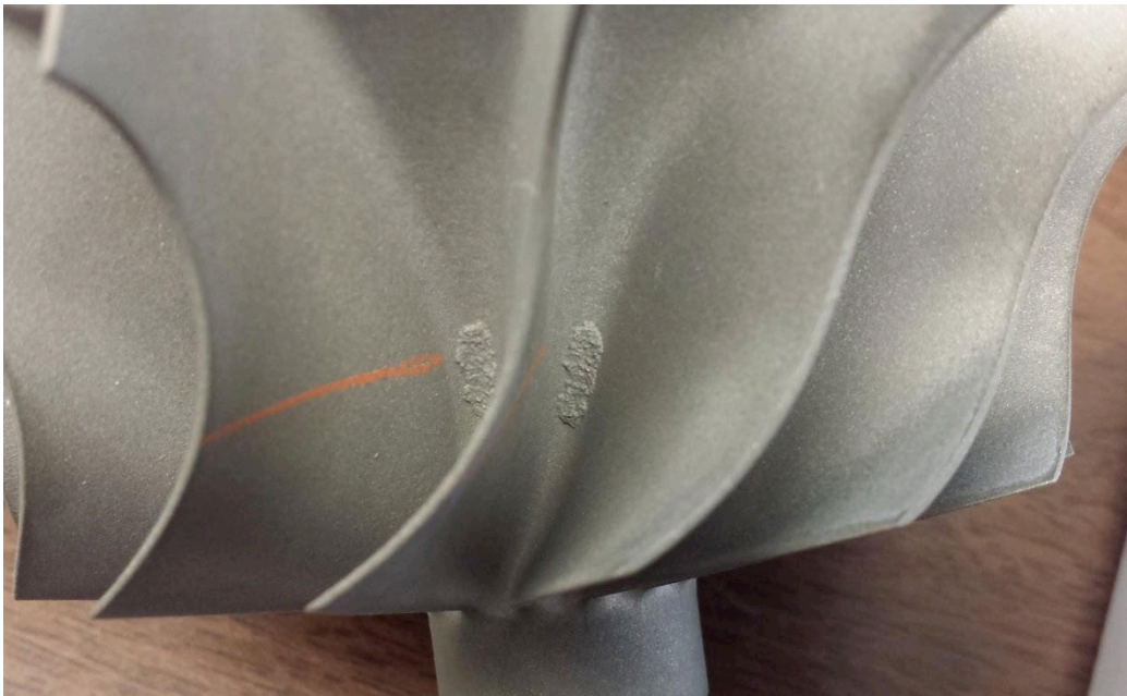
Figure 14. Defects from spalling in a cast part. Two spalling defects present on the surface of an investment cast nickel-based superalloy part. Fillet radii are common locations for these defects [PCC Structurals].
