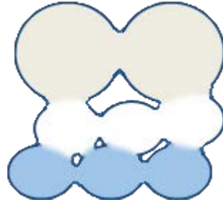
Figure 51. Diagram of the fired shell. Firing the shell allows particles to diffuse into each other, forming ionic bonds that hold the shell together more strongly than the covalent and hydrogen bonds holding the green shells.
