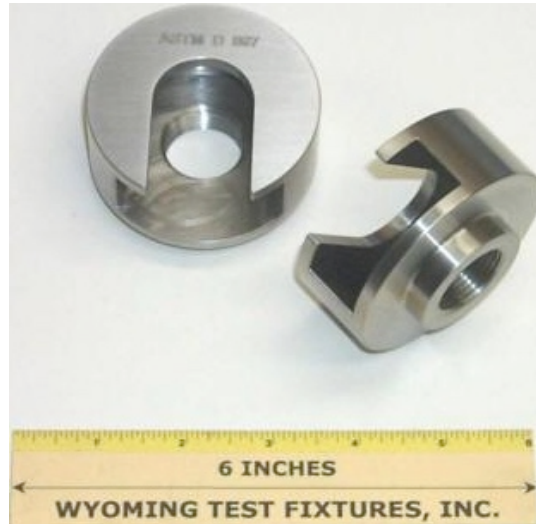
Figure 16. The fixture for ASTM D897, holds both ends of a block-adhesive-block assembly in the grips of a tensile-testing machine. The blocks are held in with a collar to even out the force on their top faces [ASTM D897].
