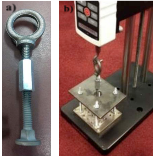
Figure 17. Fixture by Ransom & Randolph a) The initial bolt assembly to which the samples were adhered. b) The testing apparatus designed by Ransom and Randolph, with the bonded piece being drawn through a hole a suspended plate [Feffer and Holek 14, 5].
