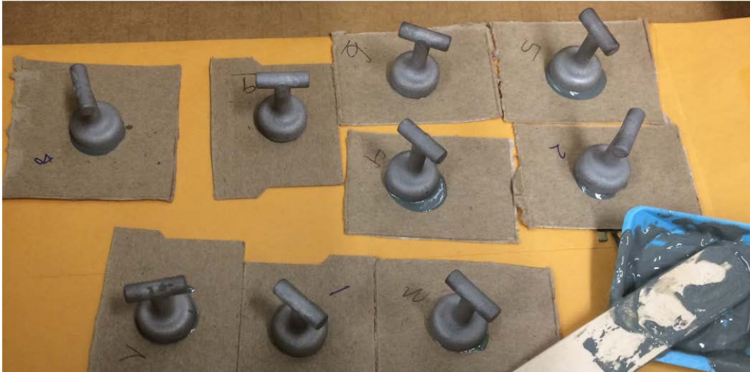
Figure 29. First button and epoxy trials on cardboard with all 9. Only 1, 6, and 9 did not have excess that spilled onto the cardboard around the button. Because they had enough extra epoxy to slide, 4 and 5 had too much.
