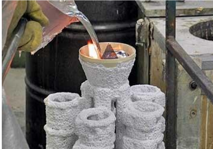
Figure 10. Pouring of an alloy into a mold. Some alloys can be poured into the mold in a standard atmosphere [Process, AlCuMet, Inc].
