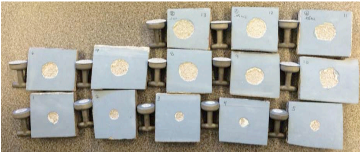
Figure 35. Tested samples from epoxy variations. The three groups of samples by name. Group A (top row) and group C (middle row) show patterns similar to previous tests. Group B (bottom row) showed a higher proportion of separation between shallower layers than the larger area samples.
