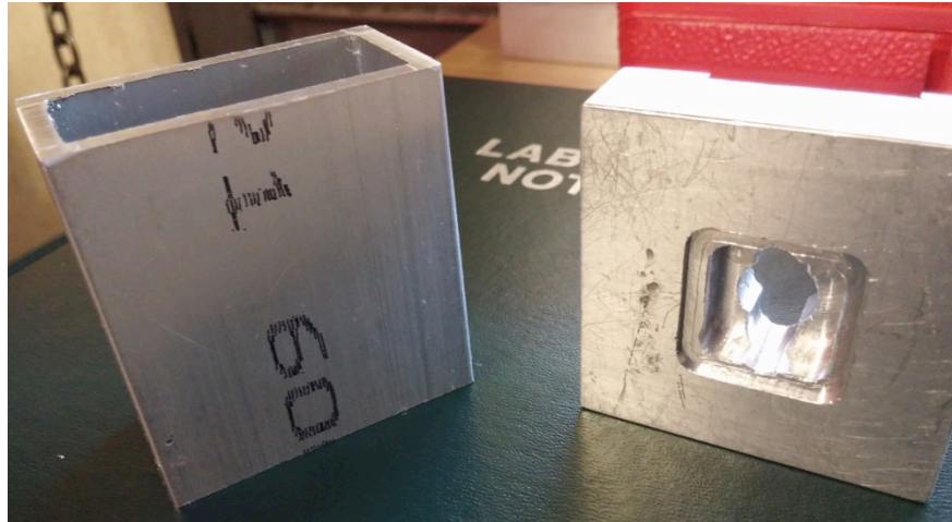
Figure 27. Machined aluminum gluing fixture parts. Some dimensions were changed to reflect the limited endmill sizes available.
