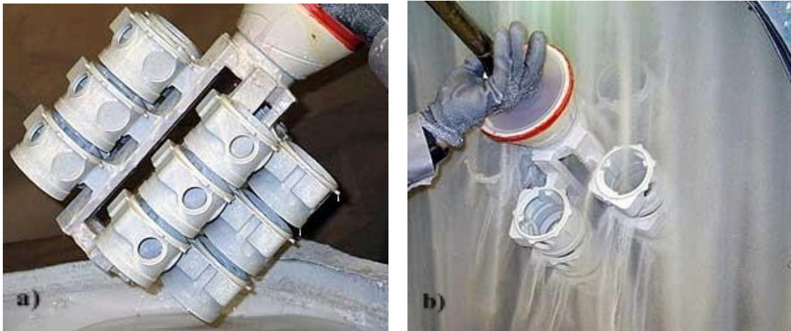
Figure 8. Slurry and stucco application a) The first and second slurry and refractory coats are applied to wax pattern trees by hand to ensure all surfaces are coated. The backup coats are applied robotically. b) A rainfall system is one of two stuccoing methods used to cover the new slurry coats with refractory particles before they are dried [Process, AlCuMet, Inc.].
