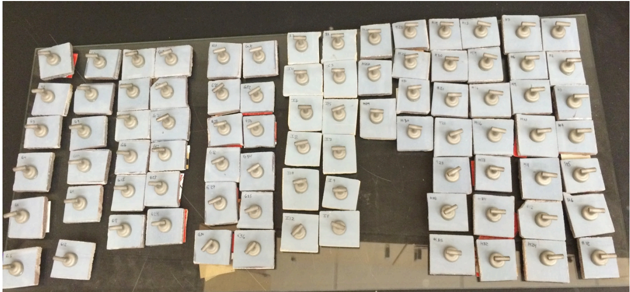
Figure 42. Leveled glass table with fully prepared samples, in the setting process.
