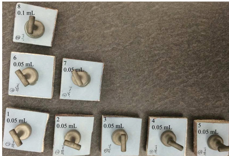
Figure 33. Modified epoxy volumes and leveling. Five of the seven buttons attached with 0.05 mL stayed put and had little sliding with no overflow, and 6th and 7th moved some. Sample 8 has 0.1 mL of epoxy, and had unacceptable overflow.
