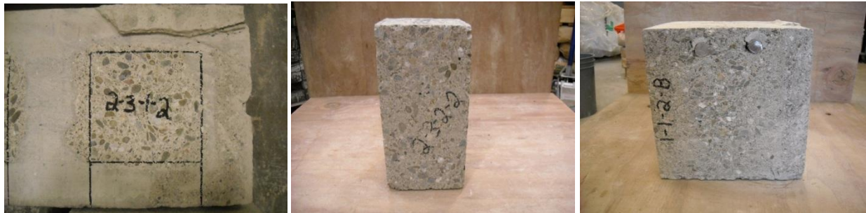
Figure 11: (a), (b), Side of Compression Specimen and (c) Consolidation Specimen
