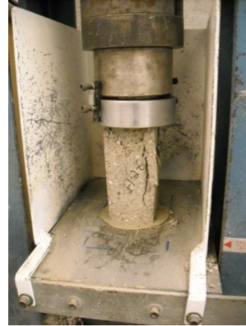
Figure 5: (a) Capping of Grout Compression Specimens and (b) Compression Testing
