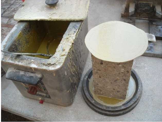
Figure 5: (a) Capping of Grout Compression Specimens and (b) Compression Testing
