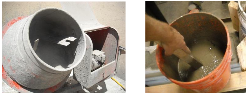
Figure 2: Grout Materials Mixing in (a) Mechanical Mixer and (b) Re-Mixing in Bucket
