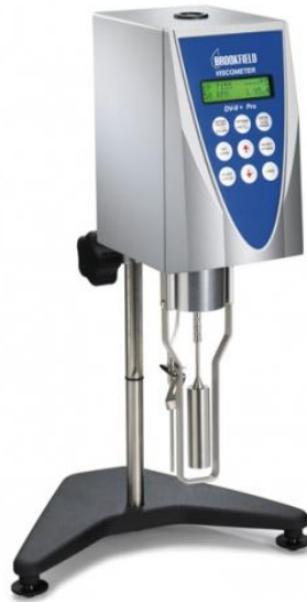
Figure 25: Brookfield type viscometer that was provided by the Food Science Department at Cal Poly
