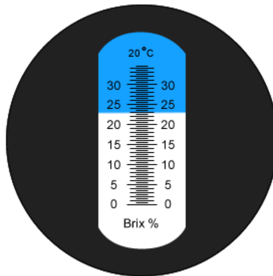
Figure 38: An example of how to use a refractometer. Place the drop of the desired juice onto the daylight pane and look into the viewing piece (Aquarium Line).
