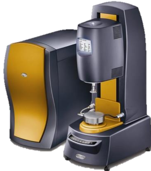
Figure 26 : Discovery Hybrid Rheometer that was provided by the Chemistry Department at Cal Poly
