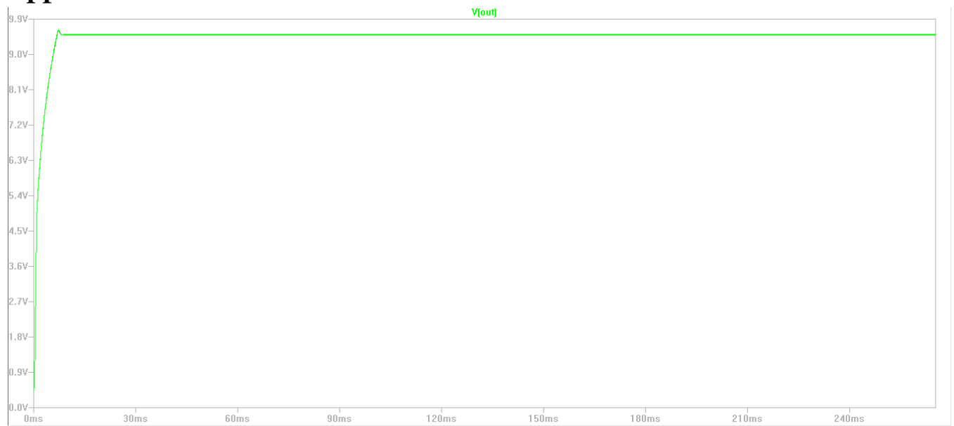
Simulation of the Buck/Boost converter: Steps up 3.7 V to about 9 V
