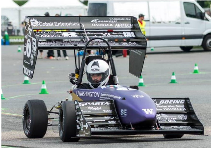
Figure 72. University of Washington's car. Note the front wing mounts coming through the nosecone, and how it allows the nosecone to maintain a continuous geometry.
