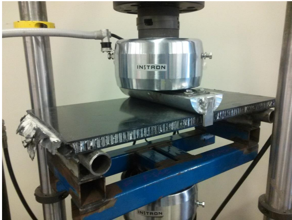
Figure 27. Long beam bend test. Safety tabs were welded onto both sides of the 4-inch diameter impactor to prevent specimens from sliding off the fixture.
