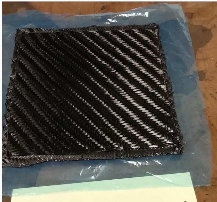
Figure S11. The tapered stack prior to application onto the monocoque. FEP was used to apply pressure to the fabric since the facesheet would not hold vacuum and bagging the entire vehicle was not possible. West Systems 105 resin and 207 hardener were applied to the fabric.
