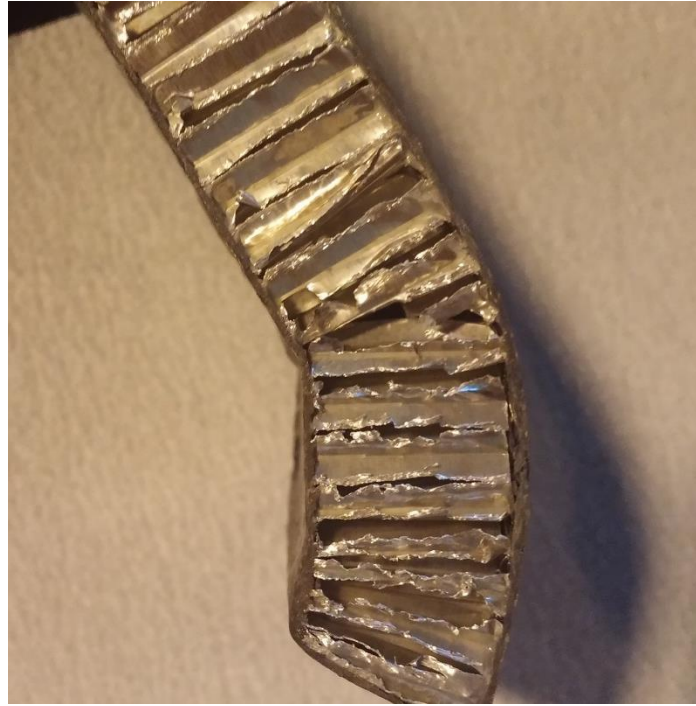
Figure 35. Core bending results from an area of simple curvature
