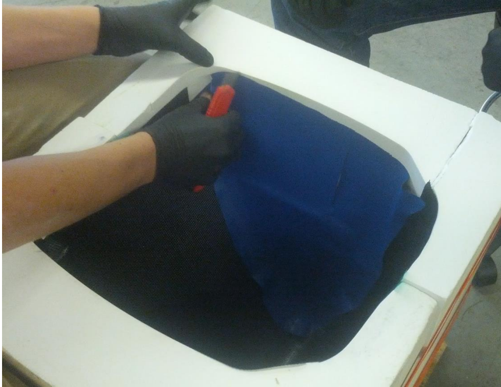
Figure 66. Laying down a ply on the side of the nosecone mold.
