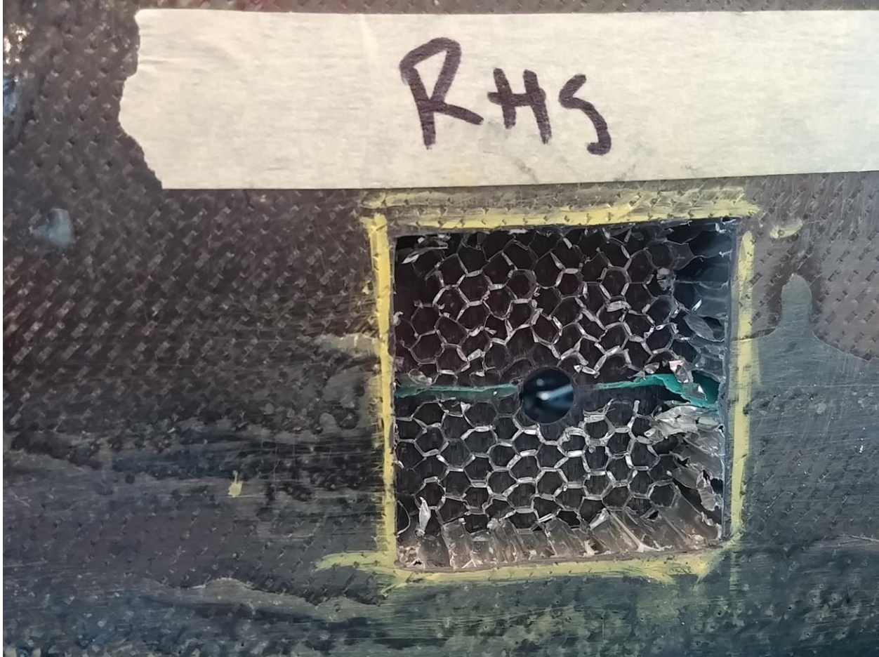
Figure S4. The core sheared loose from the inner facesheet. Balsa wood or another solution that provides higher compressive strength is highly recommended for future vehicles. Prior to bonding in a balsa wood insert, the remnants of the sheared core were removed by pulling a shard razor blade along the affected region. The blade was not pushed in an effort to reduce cutting fibers.
