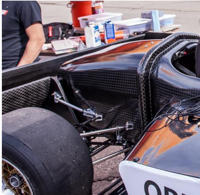
Figure 7. Global Formula Racing uses a roll hoop bonded to the outside of their monocoque. A 0.3” circular indentation was made in the mold to locate the roll bar and provide additional bonding surface area. Relocating the roll hoop to the outside of the 2015 Cal Poly vehicle would increase tubing weight from 4.2 pounds to 7.5 pounds.
