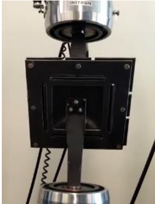
Figure 30. Off-axis pullout test.
