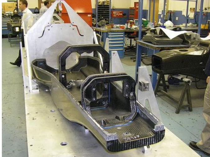
Figure 1. Formula 1 chassis, showing the use of carbon fiber and aluminum honeycomb core.
