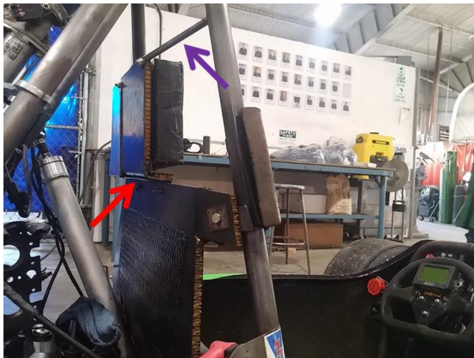
Figure 68. The cut-and-fold firewall as driven at competition. The aluminum shield on the right was added when the fuel filler neck height was increased.
