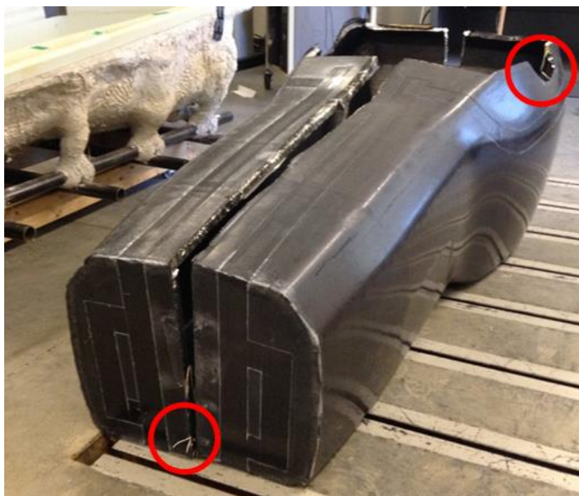
Figure 45. The two tub halves after being removed from the molds. Thermocouple locations are circled in red.
