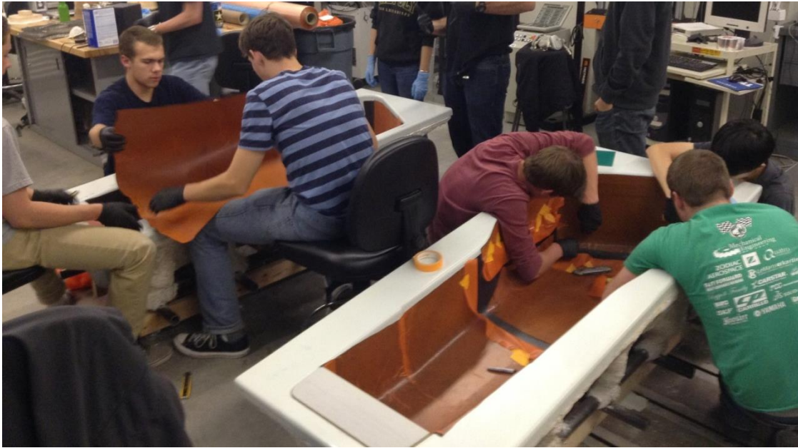
Figure 42. The team hard at work laying down plies on the tub molds. Note that multiple people are working on a single ply.
