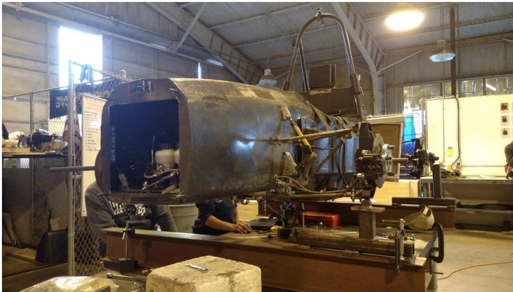
Figure 76. Torsion test front view. The front right upright is resting on a solid steel cylinder, while the front left upright is instrumented with a dial indicator and left unconstrained.
