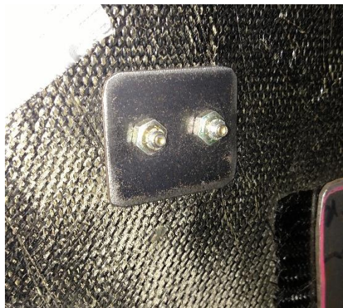
Figure 63. Backing plates used for the upper suspension mounts. Sizing was based off of perimeter shear testing results.
