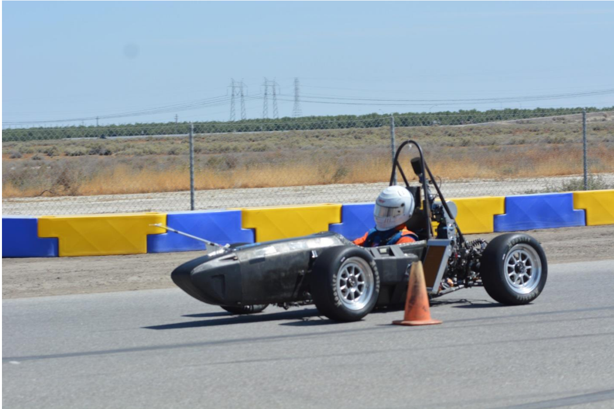
Figure 74. The car rounding a cone at the Buttonwillow Raceway kart track where a combination of curbs, fast sweepers and medium-speed banked corners provide loadings somewhat higher than those expected at competition. These loadings quickly failed the core behind the rocker mounts where balsa wood was not present.
