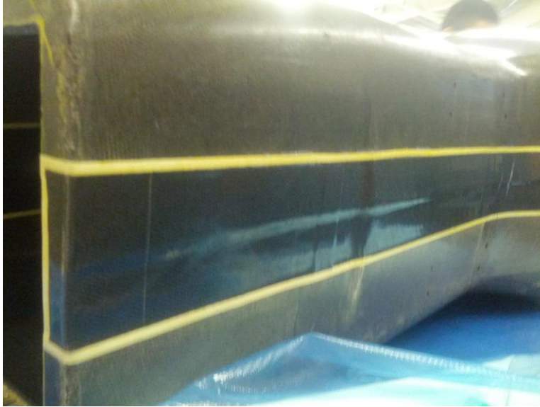
Figure 50. Carbon prepreg strap joint used to transfer load between the two tub halves.
