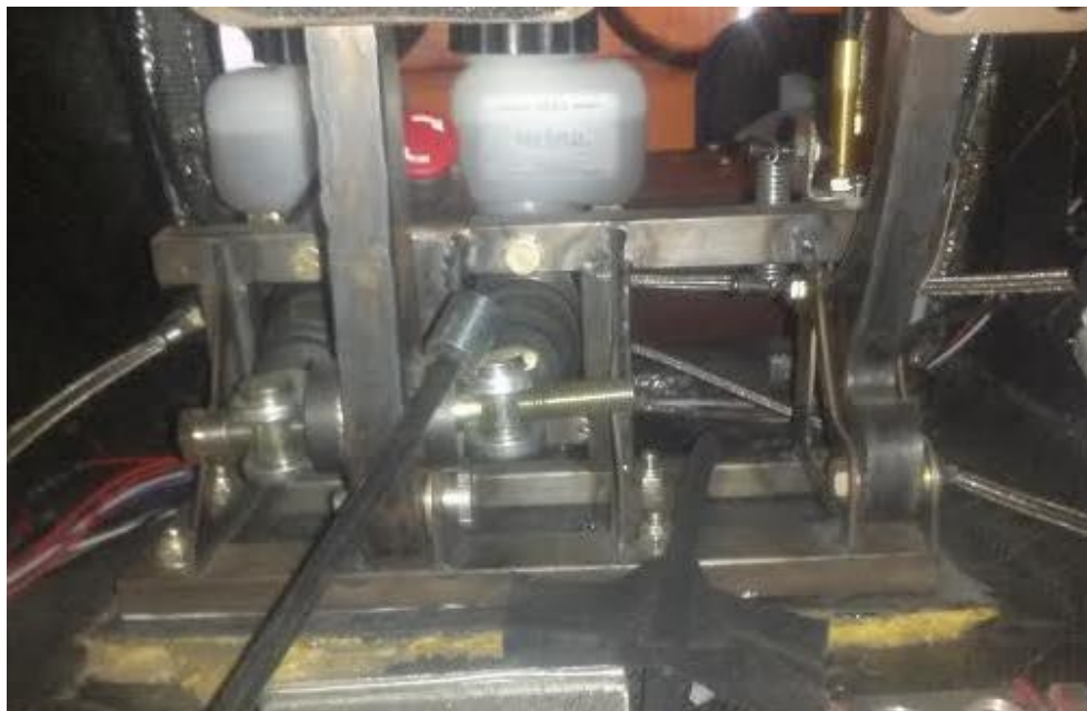
Figure 57. The resin and chopped fiber shim can be seen under the pedal-box. Graphite was added to the slurry to give it a black color. Remnants of yellow damming tape are visible along the periphery of the shim.
