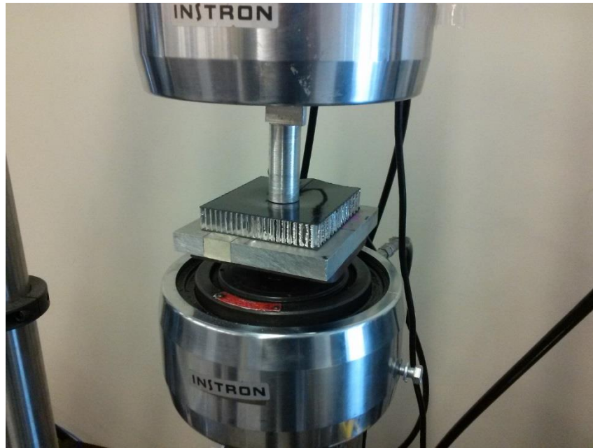
Figure 29. Perimeter shear test setup
