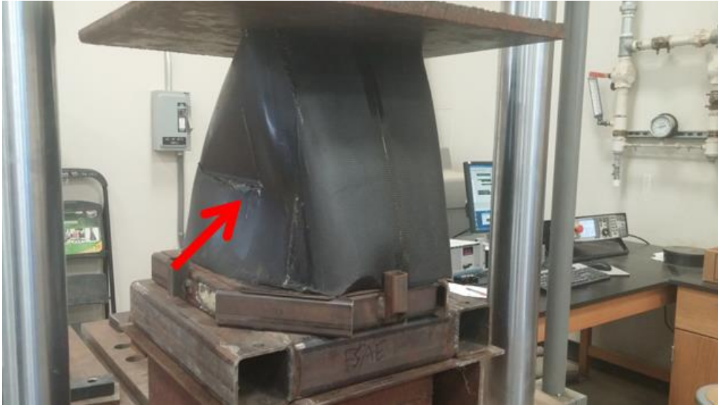
Figure P1. Nosecone crush testing revealed the failure mode to be fiber bending stress concentrations created by the wing mount flat sections (indicated with red arrow). Eliminating these flats or providing additional localized reinforcement would reduce the overall weight of the nosecone.
