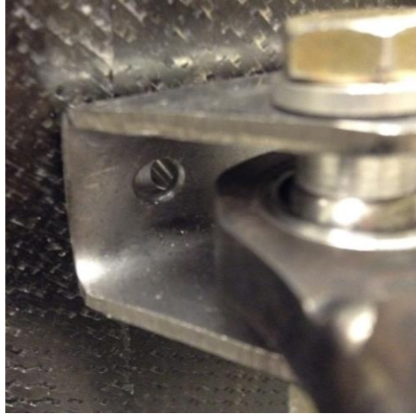
Figure 47. Mismatch between the suspension bracket holes and tub inserts required additional machining on the brackets in order for them to fit.
