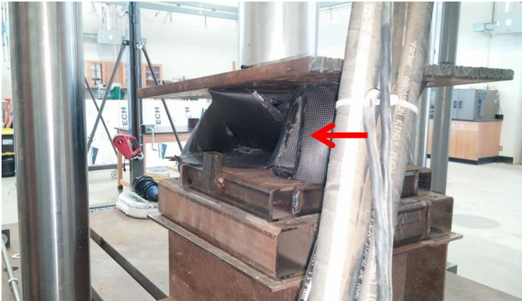
Figure P4. The recesses for the bolt/attachment flanges (one of four shown with the red arrow) held nearly 775lb of force over 4" total of travel. This value could be improved by bolting the flanges onto the fixture as they began to tilt prematurely. The geometry's resistance to buckling and ability to raise load-holding capability far into the displacement spectrum can be exploited by future teams to help meet energy requirements.
