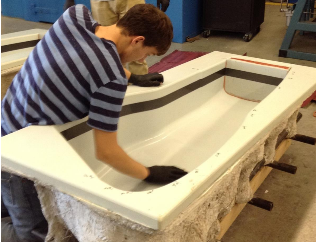
Figure 41. Tub mold with nylon strap. Note that the nylon strap is applied right inside the scribe line, so the recess would be along the edge of the tub when joined. Release agent was applied after the nylon stripping was added.
