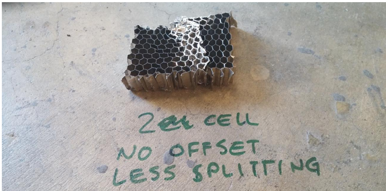
Figure Y2. Another example of core-splicing using a third piece hammered into the joint. Not offsetting the third piece kept the most cells intact. This was the best way FMD found to execute this method.
