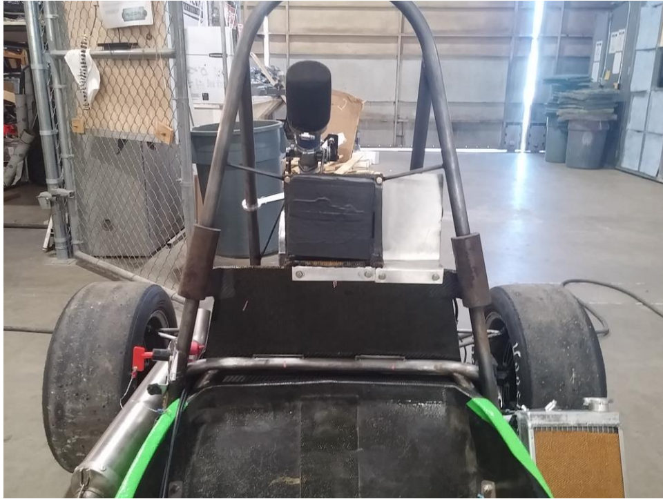
Figure 68. The cut-and-fold firewall as driven at competition. The aluminum shield on the right was added when the fuel filler neck height was increased.
