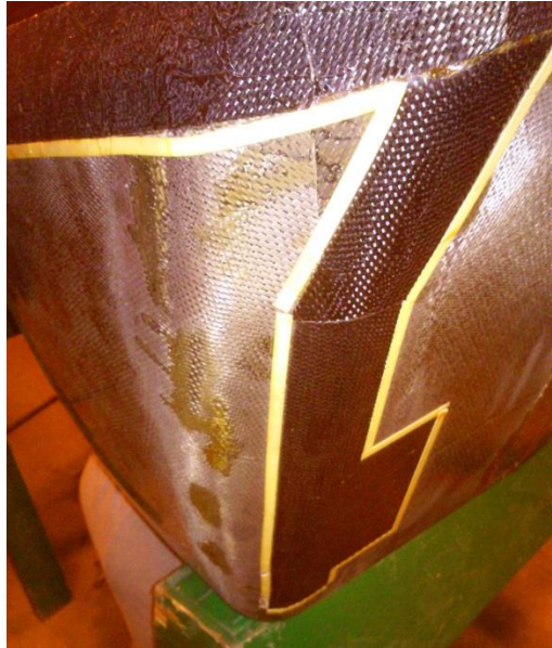
Figure 58. The darker repair patch runs along the length of the subframe mounting surface, creating an uneven step that prevented flush mounting.
