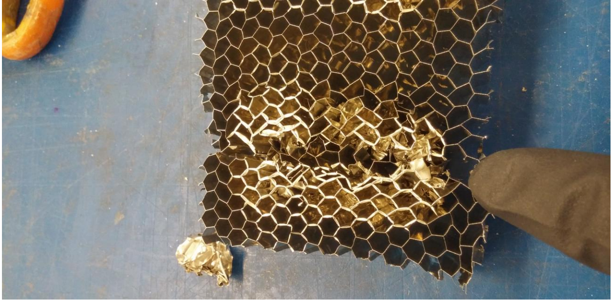
Figure Y3. This section showing the bottom side shows poor joining at the seam. Aligning the smashed-down pieces cells reduced this splitting effect.
