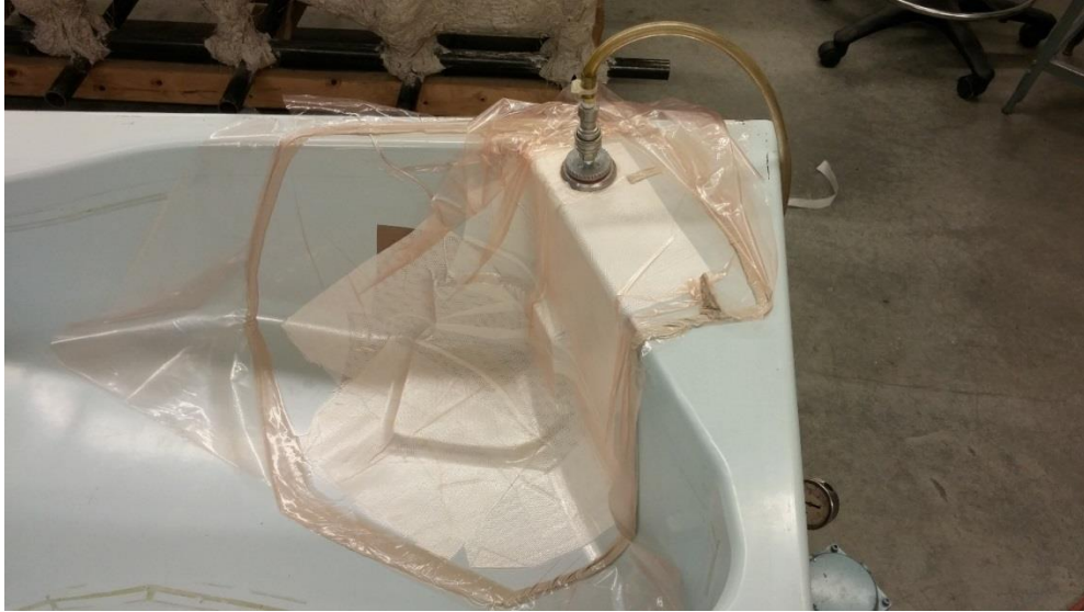
Figure 34. Sample blob layup in a region of the tub mold with complex curvature.
