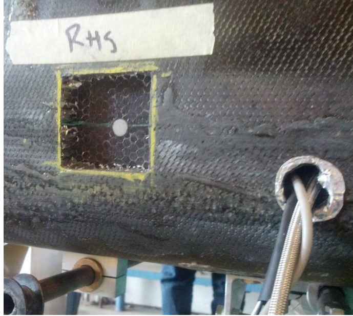
Figure 61. Location and size of repair section at front rocket mount. Note how both the outer face sheet and aluminum core have been cut out, but the inner face sheet was not.
