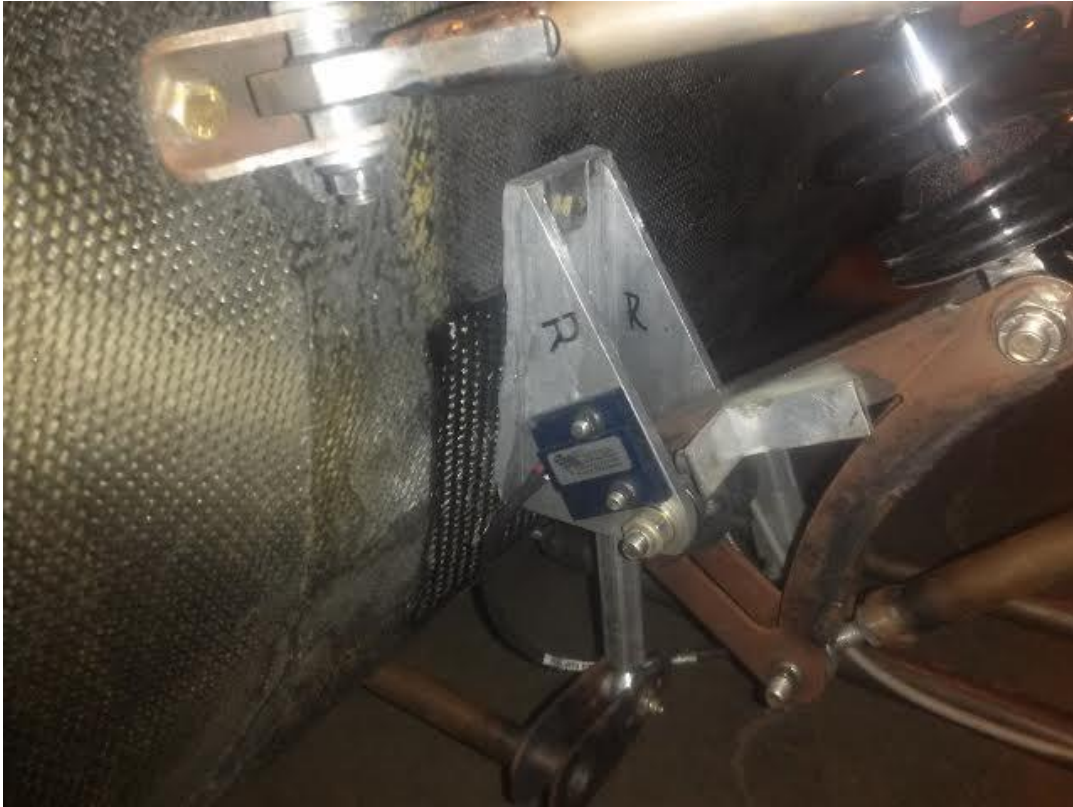
Figure 60. Rocker mount with cured aluminum paste shim. The grey aluminum paste shim is visible where the bracket meets the tub. The paste shim appears thicker than it actually is due to leftover residue adhering to the side of the bracket.
