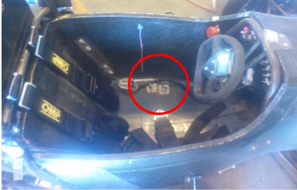
Figure 6. Lap belt and anti-submarine harness attachment locations. This bracket arrangement is replicated on both sides of the cockpit floor.
