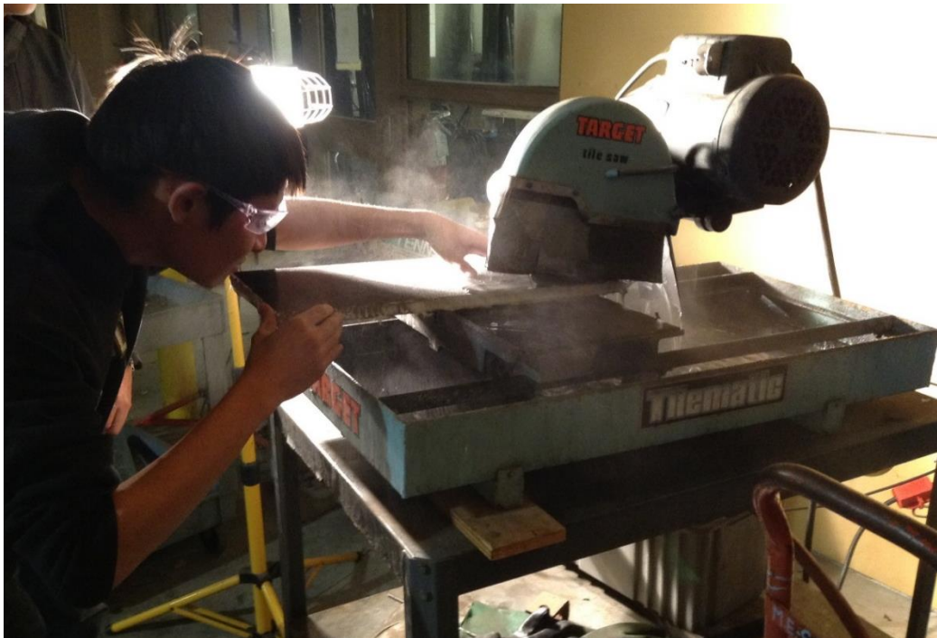
Figure 40. Test panel being cut on the tile saw.
