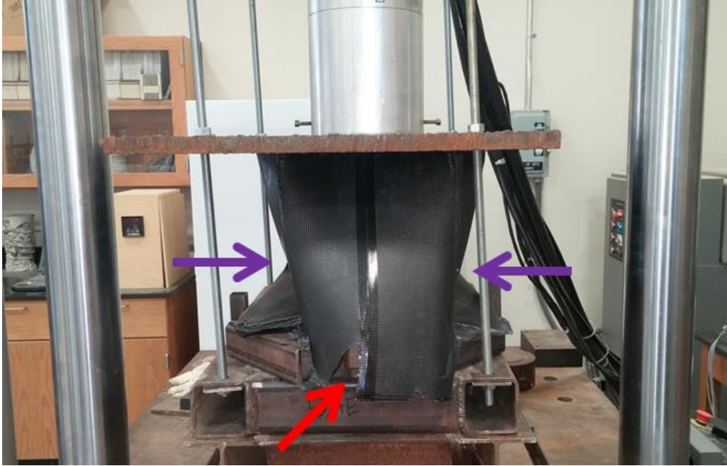
Figure P3. With increased displacement of the impact head the nosecone broke past the rectangular tube (shown with red arrows) and the edge protruding beyond the fixture lost ability to carry significant load. The primary failure mode continued to be the wing supports at this stage as indicated by the purple arrows. Note that the threaded rod was only used for repositioning the test machine head, not during dynamic testing.
