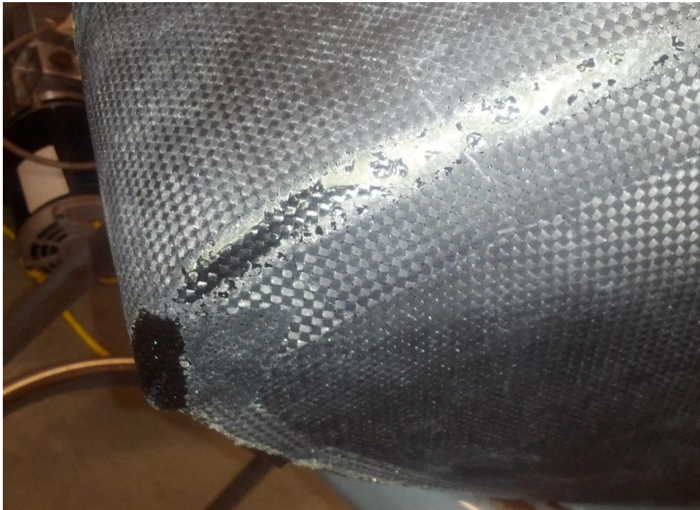
Figure 73. Picture of nosecone dry spots, most likely caused by carbon bridging hindering vacuum pressure from pushing carbon against mold surface.
