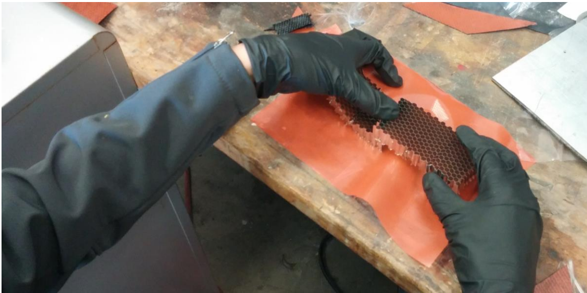
Figure Y6. Simply overlapping two pieces and hammering down was unpredictable. Some samples joined exceptionally well and others poorly when the top piece moved downward at an angle.
