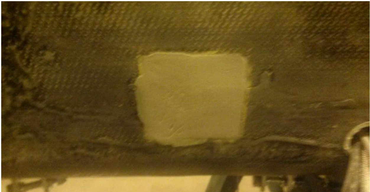
Figure S7. Following preparation of the balsa plug, resin and microballoons were mixed to a frozen-yogurt consistency (to allow for flow into the core). An excess amount of the resin and microballoons were inserted into the cavity to reduce potential voids in the dried slurry. The excess protruding beyond the facesheet was then wiped flush before curing.
