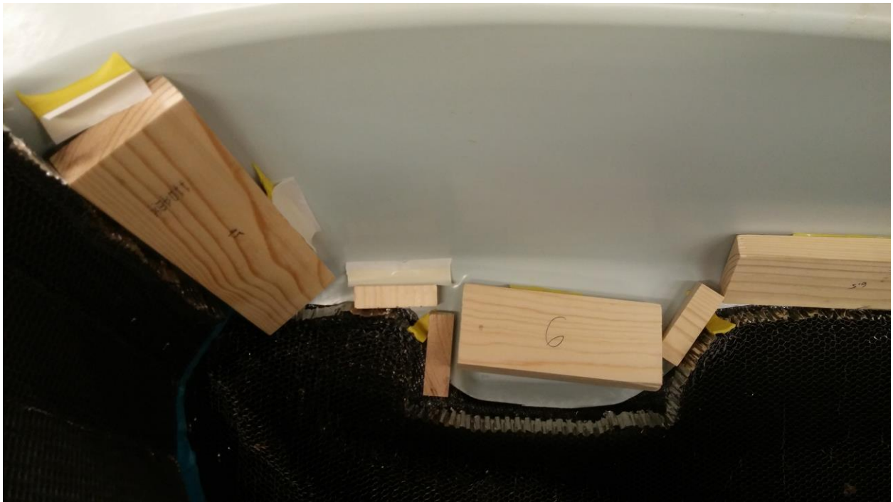
Figure Y14. Wood was inserted at the edges of the core by the cockpit opening (shown) and all other edges (not pictured) to prevent core from crushing while under vacuum in the debulking and cure cycles.
