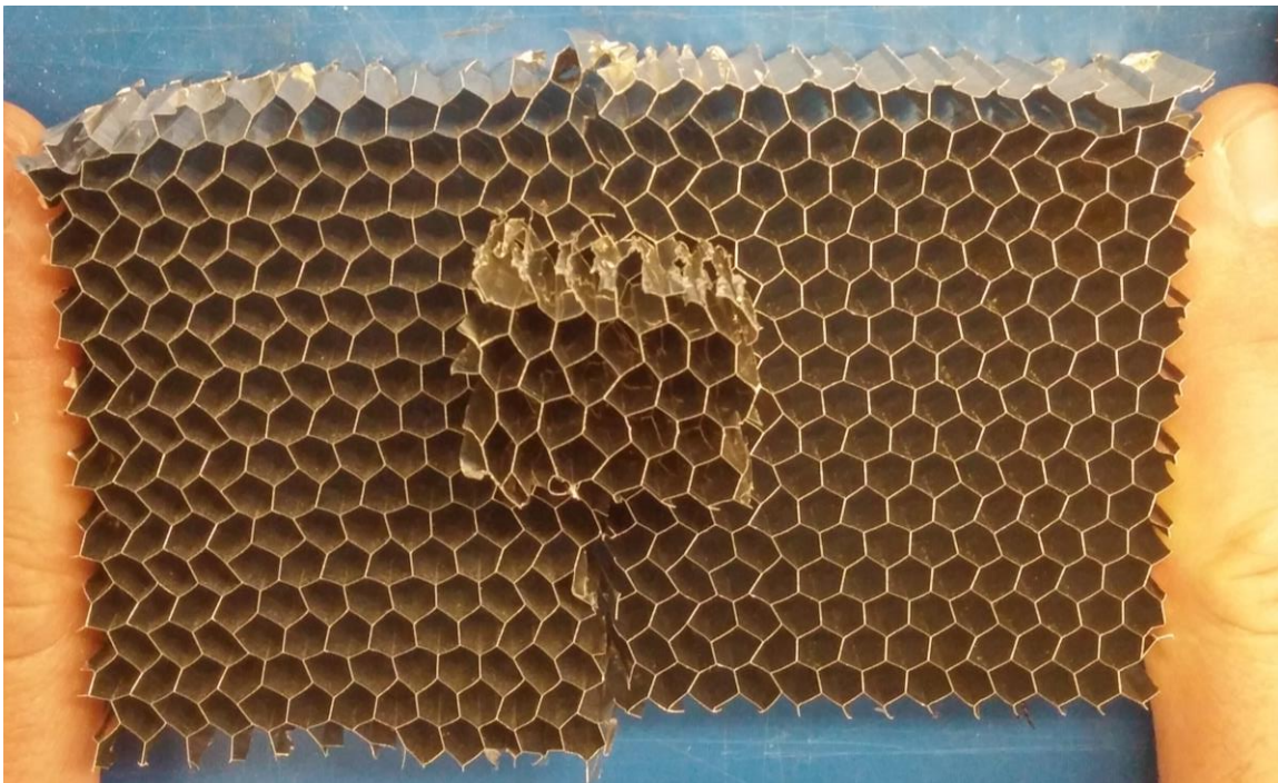
Figure Y4. Two pieces of core butted together with the third piece ready to be smashed into the joint.
