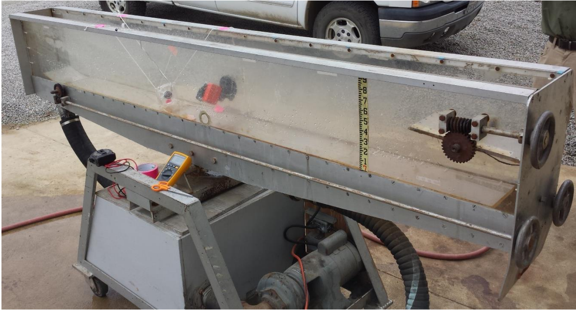
Figure 24: Fan Blade Speed Test Flume
