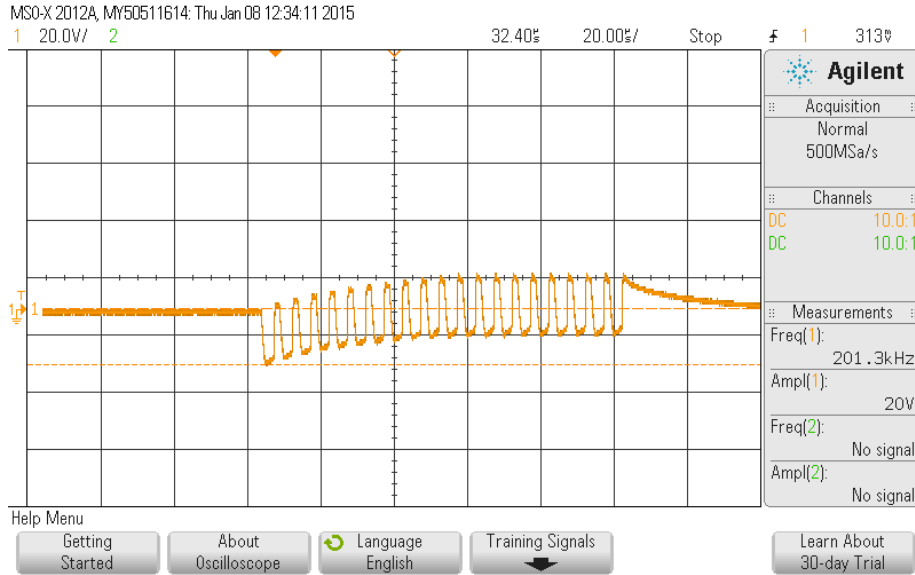
Figure 17: Fish-Finder Transmit Signal
