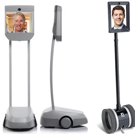
Figure 1: Two commercially available telepresence robots: Beam Telepresence Robot (left) and Double Telepresence Robot (right)
