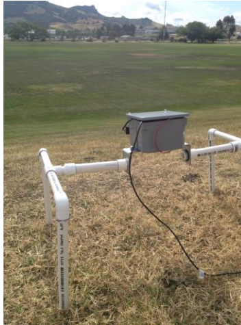
Figure 34: Testing with the sensor beam directed parallel to the slope of a hill.
