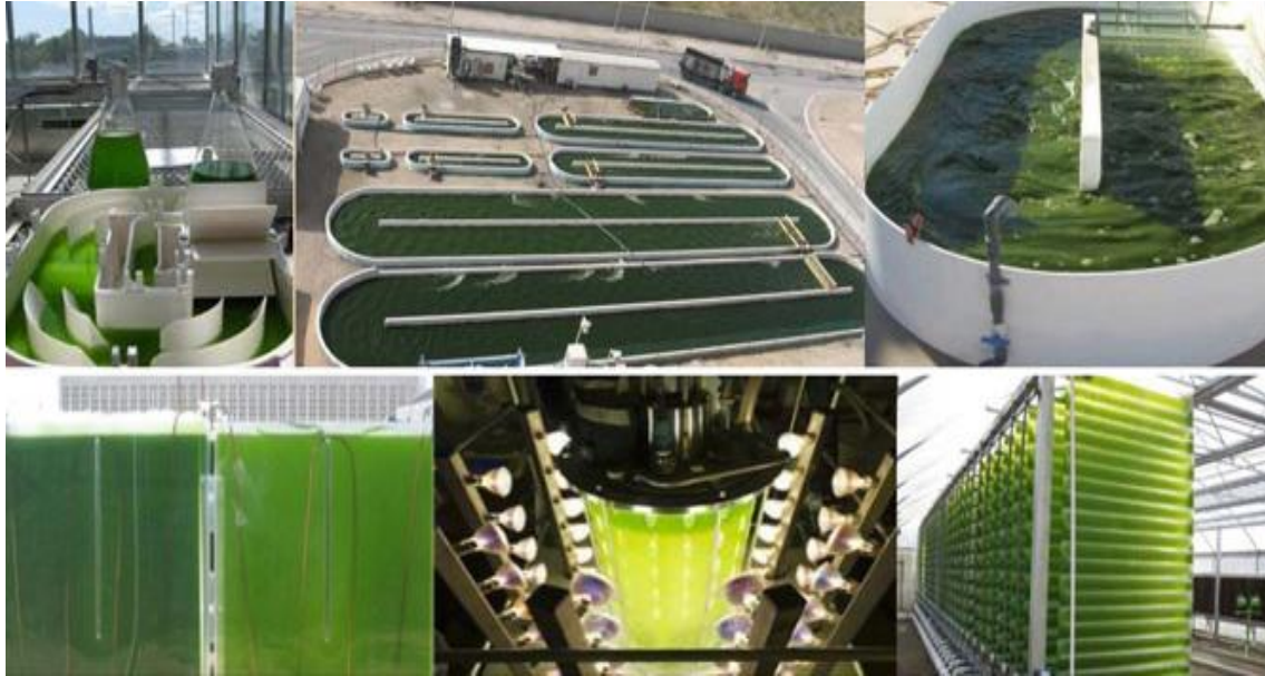
Figure 4: Different types of microalgae culture system. The image shows the open culture systems in upper quadrants, while in lower quadrants the closed culture systems or photobioreactors appear.
