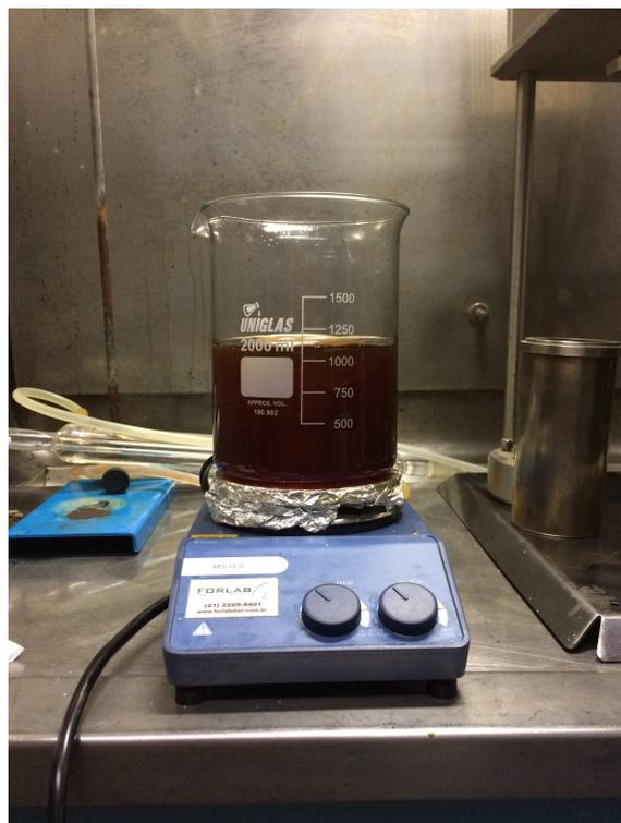
Figure 4.11: Heated magnetic stirring apparatus used to dry the WCO
