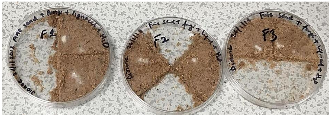
Figure 4-8: Specimens were each divided into four sections disrupting the already formed total surface mycelia layer. These images were taken in the process of transferring each quadrant into a fresh petri dish which also provided sufficient test samples for subsequent tests
