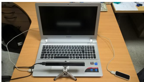
Fig. 3. The test environment with Eye Tribe Tracker and Leap Motion Controller (source: own edited)
