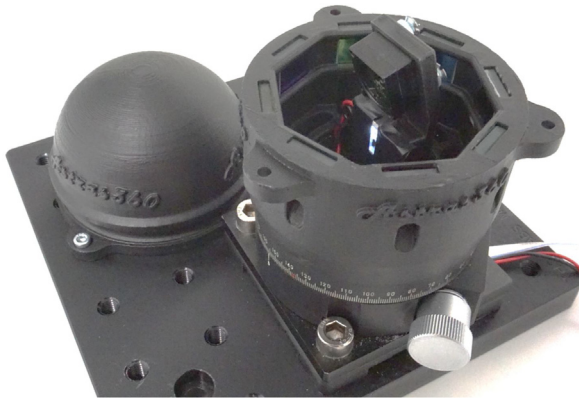
Fig. 9. Photo of the characterization prototype featuring a rotary mount. During the tests, the dome was closed in order to prevent the external light to reach the image sensor. The parts were black painted to avoid unwanted light reflections.
