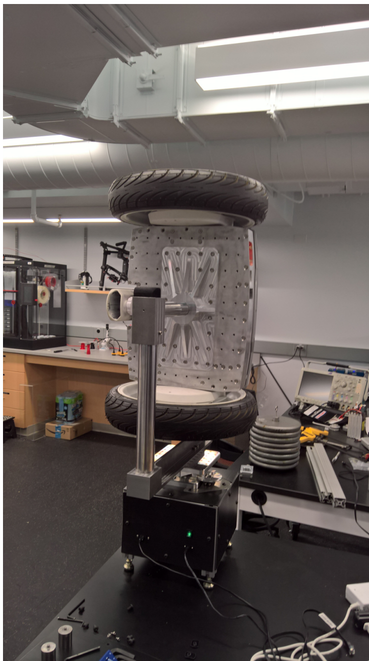
Figure 2.22: Picture of the segway vehicle on the inertia test bed.
