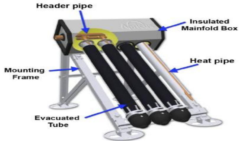
Figure 1.3: Evacuated tube collector [7]
